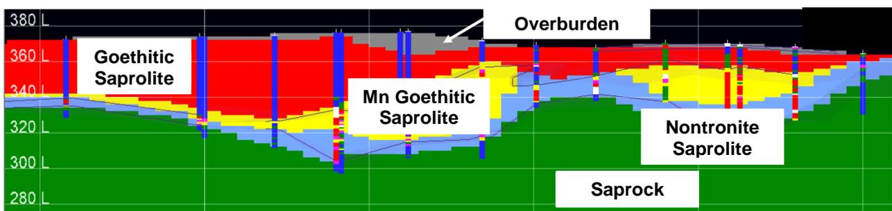
Figure 3 – Geological domain model typical cross section
