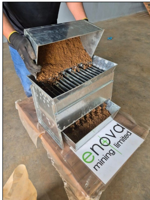
Figure 7: Enova professional geologist sub-sampling by using riffle splitter
