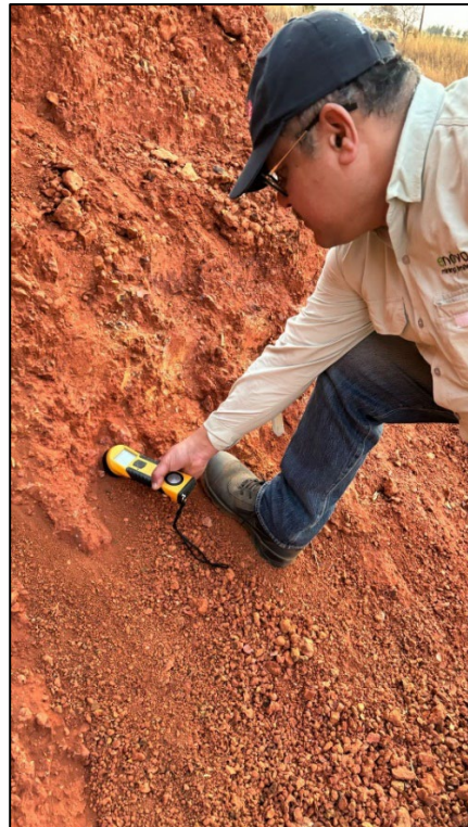
Figure 10: Competent person is assessing the magnetic susceptibility of volcanics on the outcrop
