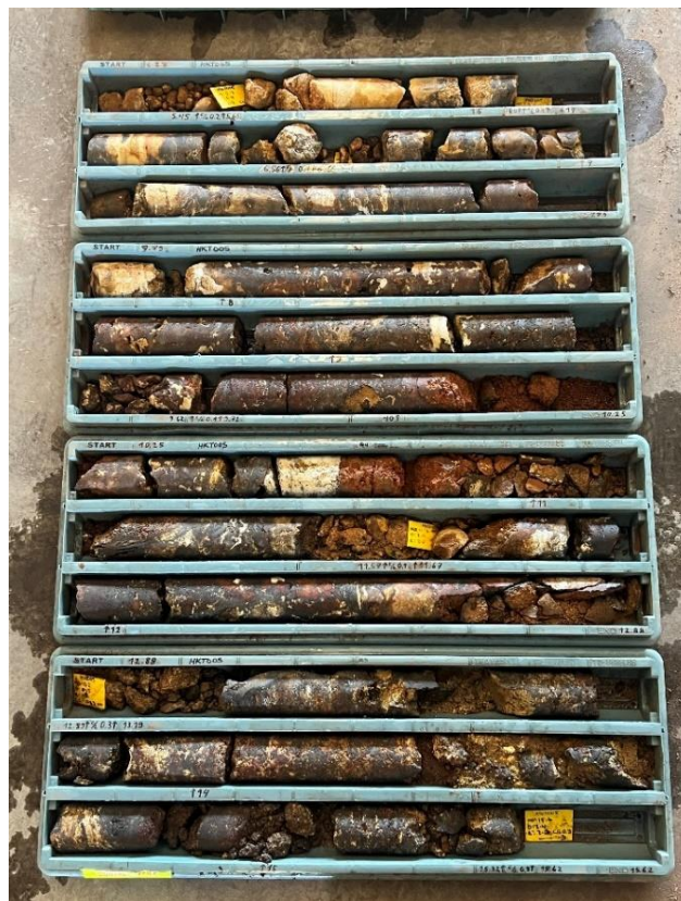
Figure 6: Hendeka PQ3 diamond drill core samples from hole HKT005 were included in a metallurgical composite sample.
