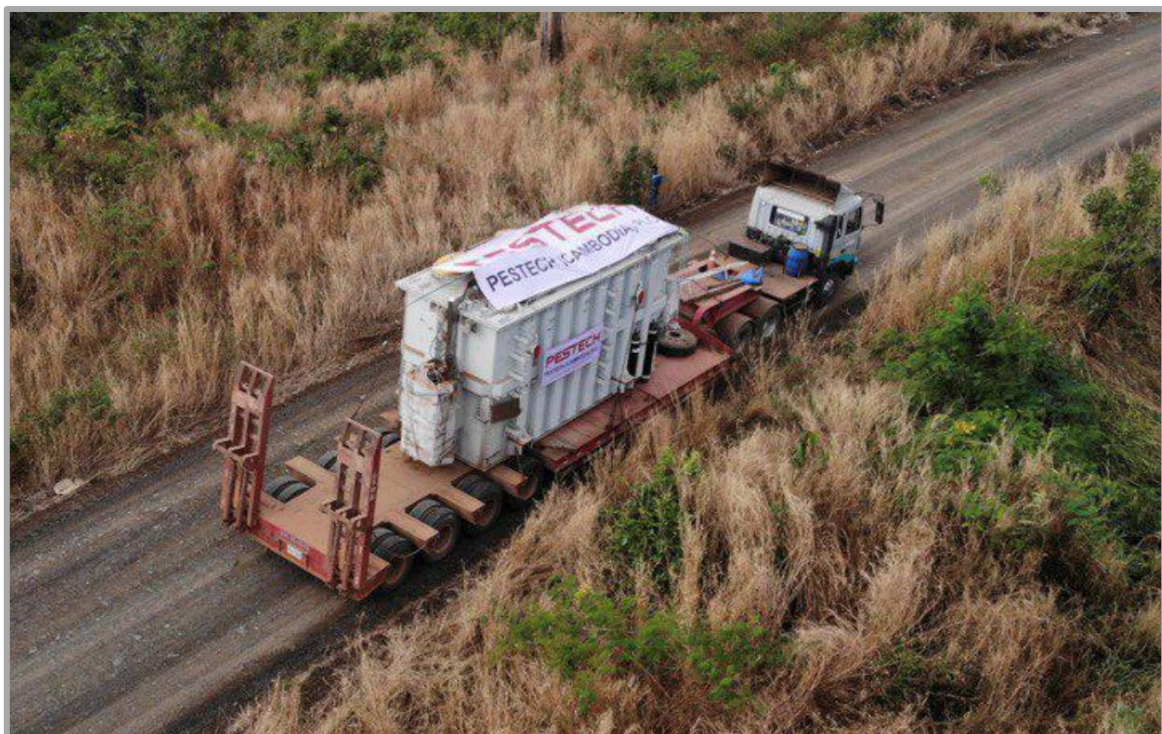
Figure Two | Transformer transported to site
