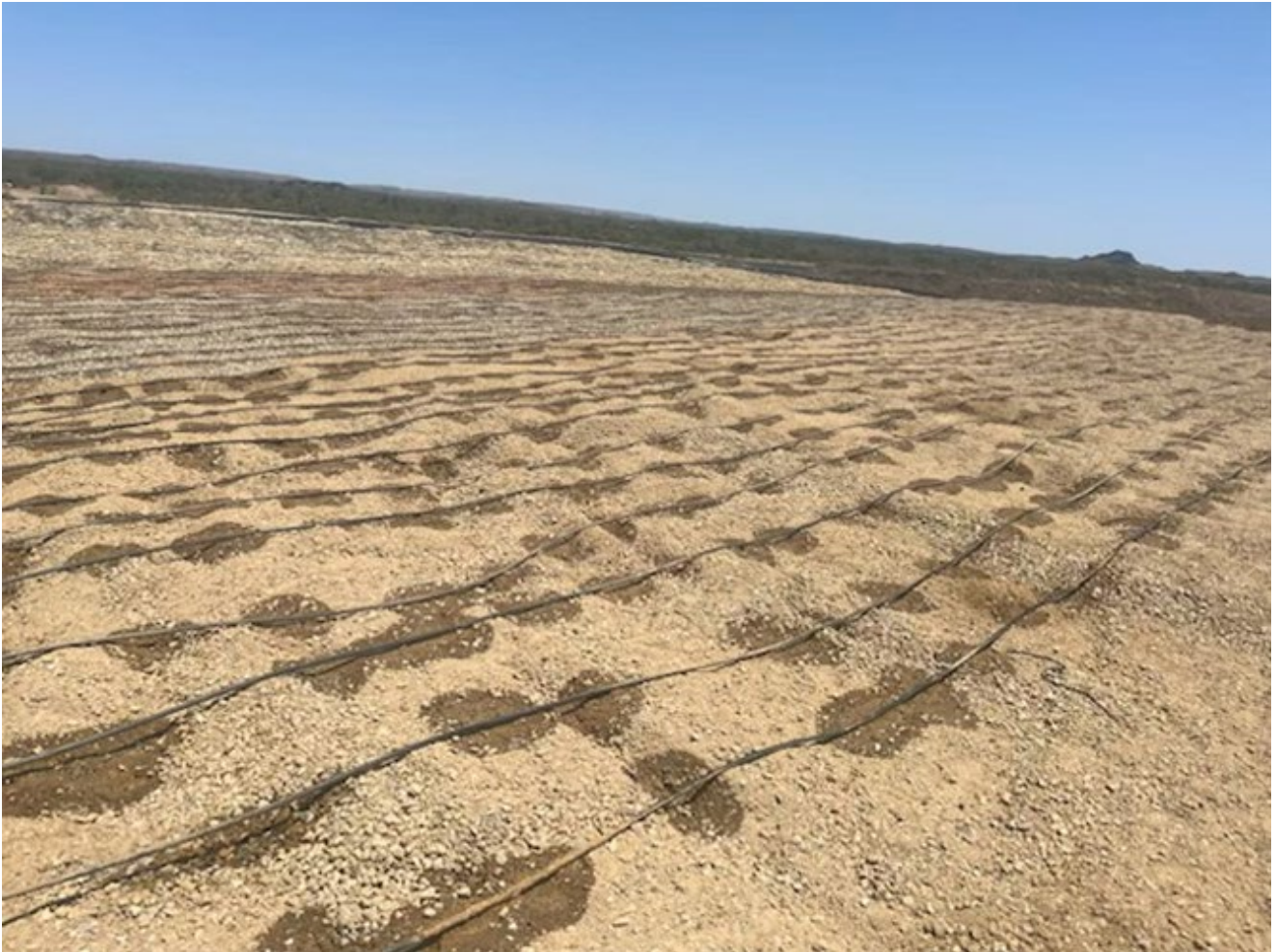
Figure 2. Leach pad 5 under irrigation on 8 October 2024.
