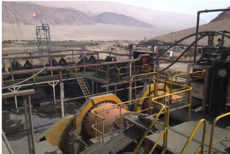
Figure 3: San Santiago Plant flotation circuit.
