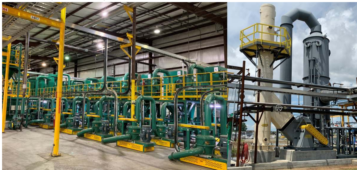
Figure 4: Installed plant at Vidalia. Left: Milling, Right: Environmental scrubber
