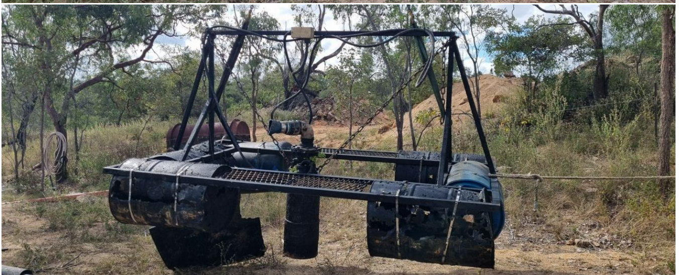
Removal of PC Dam Raw Water Dam Pump (07-PP-05) and Pontoon for Inspection and Refurbishment
