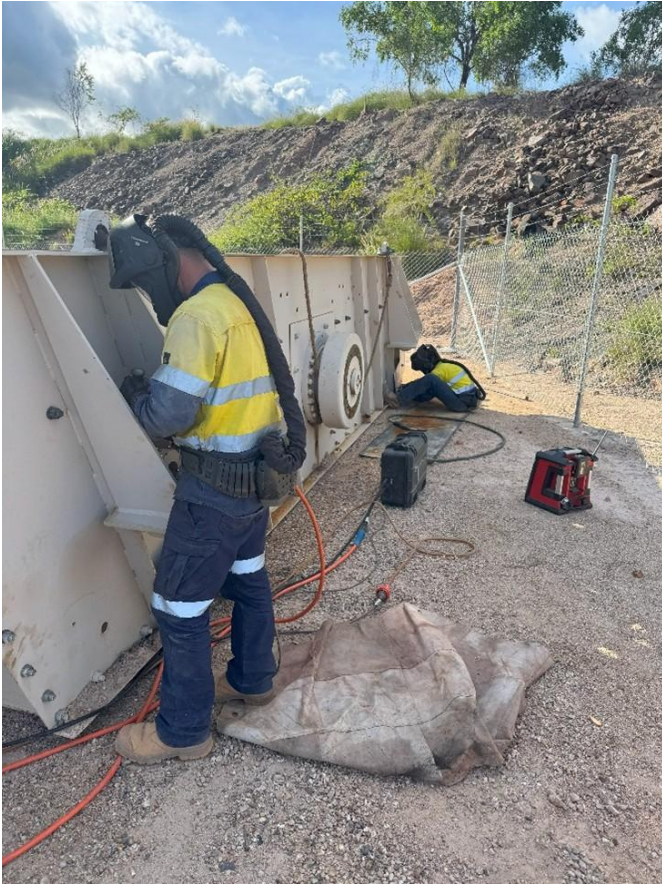
Completed repair of Shaker screen with new modification works
