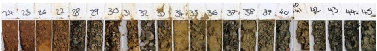
Photo 2: NMWBAC22-256 Target 4.1 24-45m Hematite altered quartz porphyry (8m @ 4.00g/t Au within 21m @ 1.69g/t Au from 24m)
