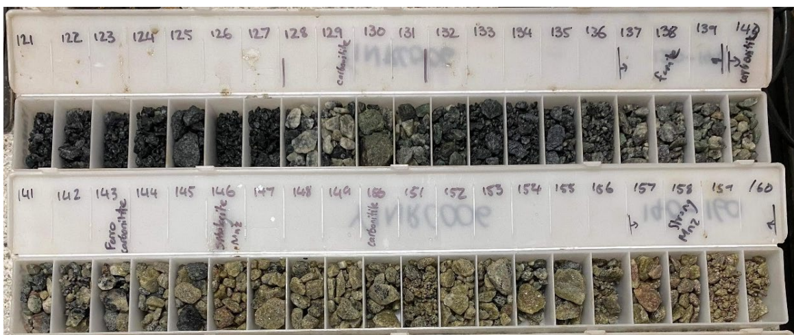
Figure 9: Chip tray from YINRC006 showing dark fenitic alteration grading into two mineralised fresh ironstones (ferrocarnatite) from 127-131m and 139m-160m.
