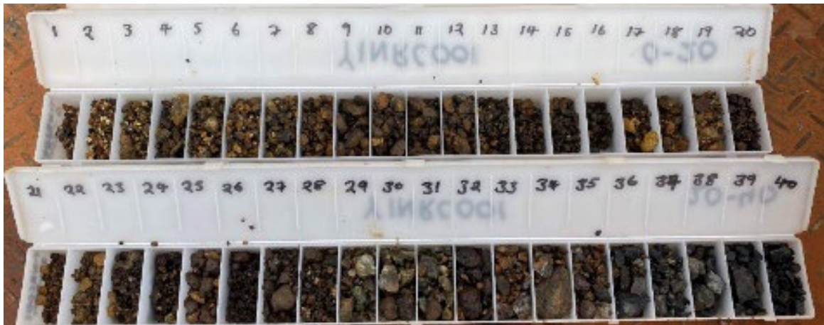
Figure 8: Chip tray from YINRC001 showing mineralised oxidized ironstone from 1-34m and grading into dark fenitic alteration.
