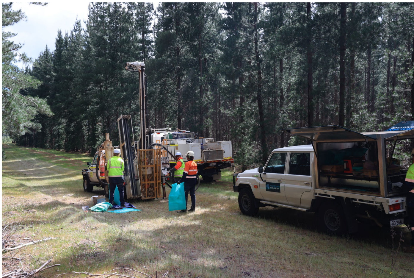
Figure 1 – Aircore drilling in commercial forestry plantations near Koppamurra Resource in October 2023
