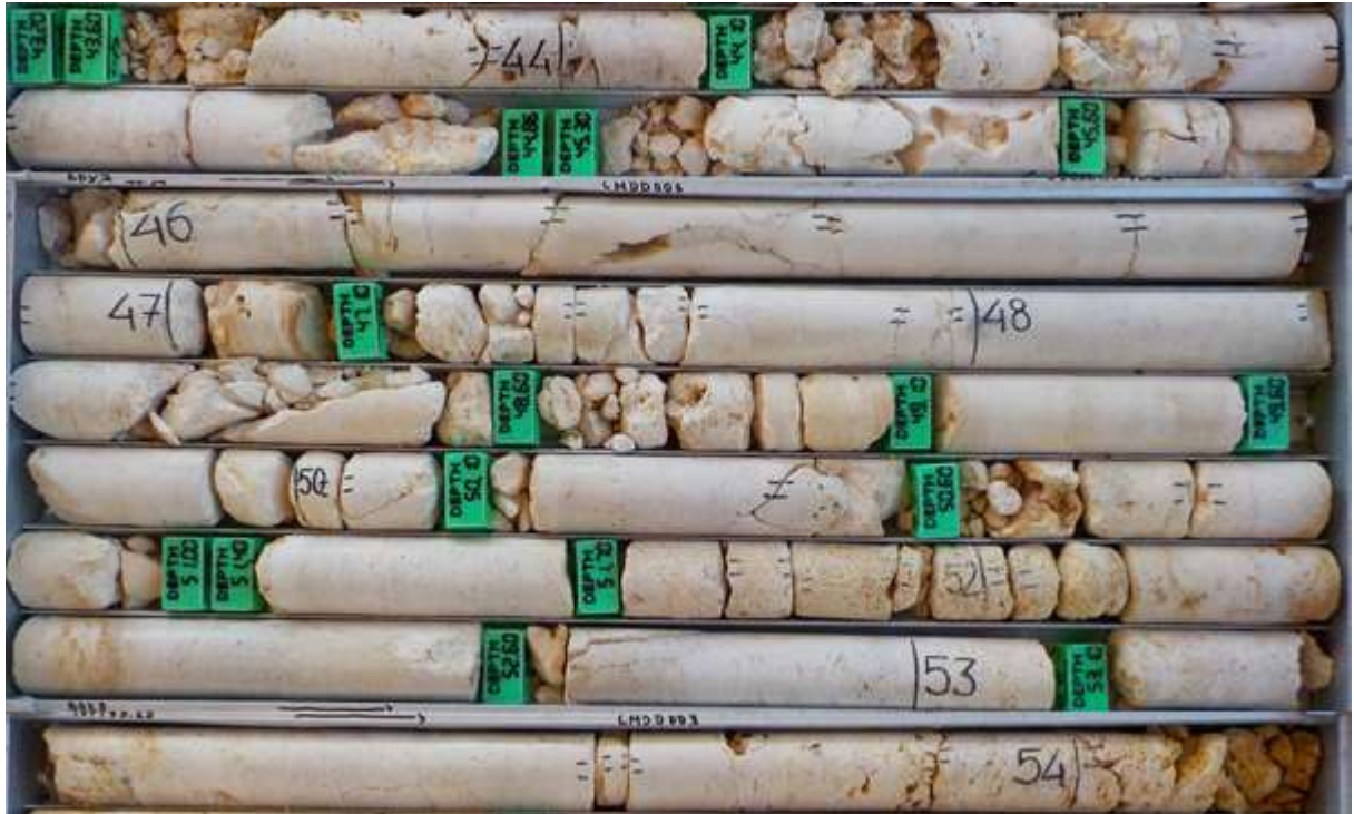
Fig 10 - “VERY HIGH” purity core (CMDD003), 43.60 to 53.74m, weighted average 55.45% CaO (98.97% CaCO 3 Limestone)
