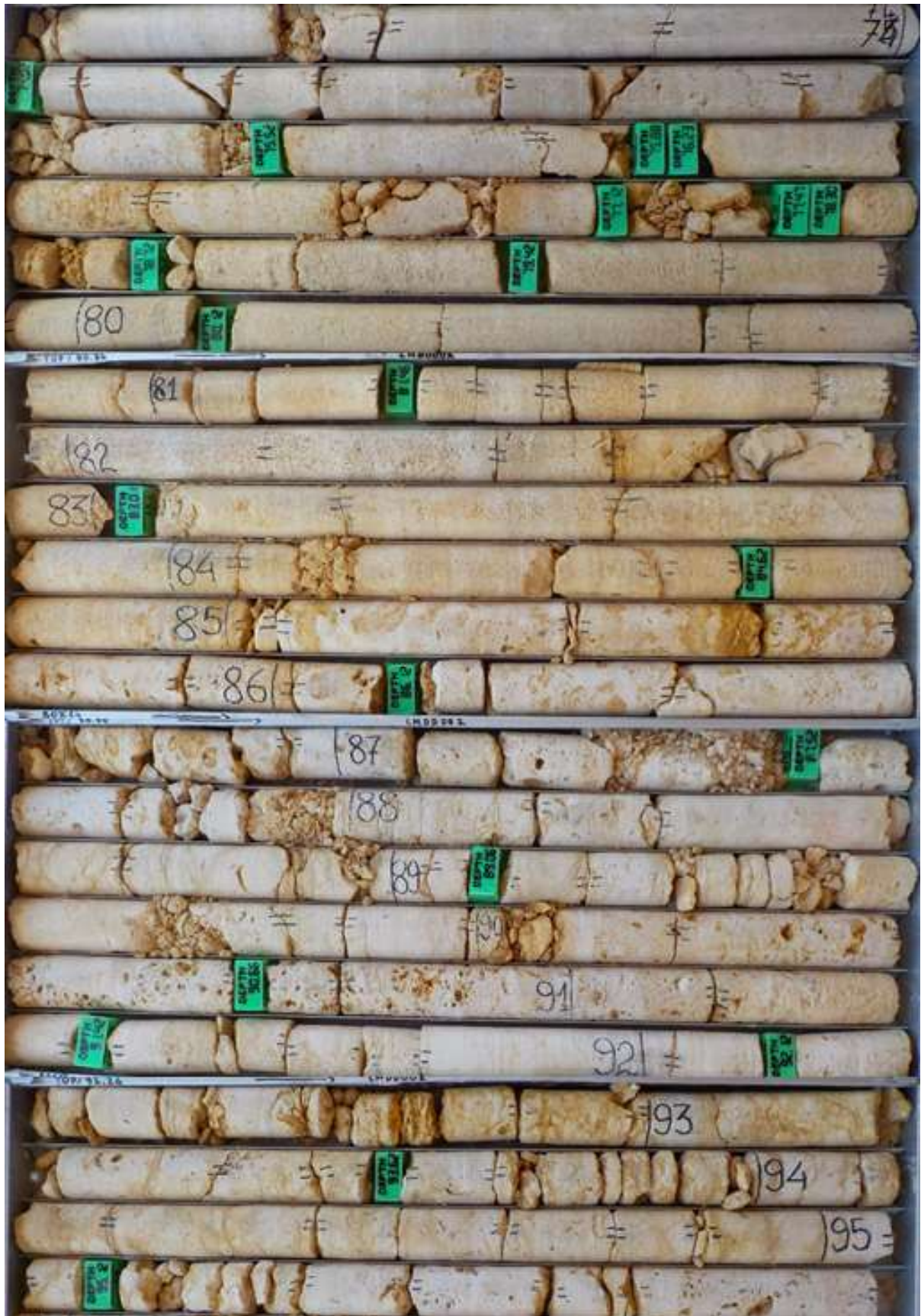
Fig 12 – “MEDIUM” purity core (CMDD002), 74.70 to 95.93m, weighted average 53.67% CaO (95.80% CaCO 3 Limestone)
