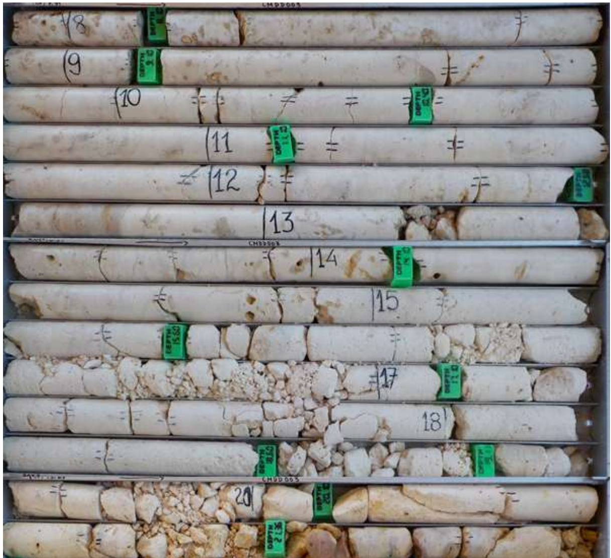
Fig 11 – “HIGH” purity core (CMDD003), 8.00 to 21.30m, weighted average 54.92% CaO (98.04% CaCO 3 Limestone)
