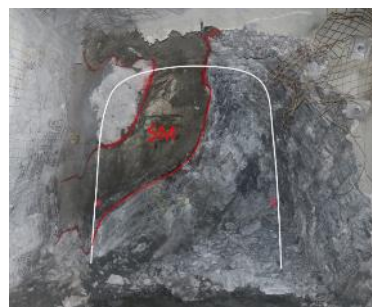
110 south ore drive (4.5mW x 4.5mH) with a face grade 2.7%
