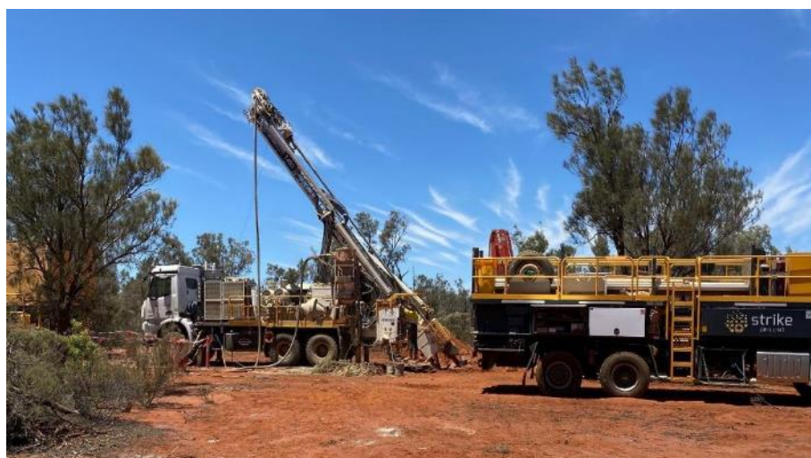
Emu Lake Reverse Circulation (RC) Drilling
