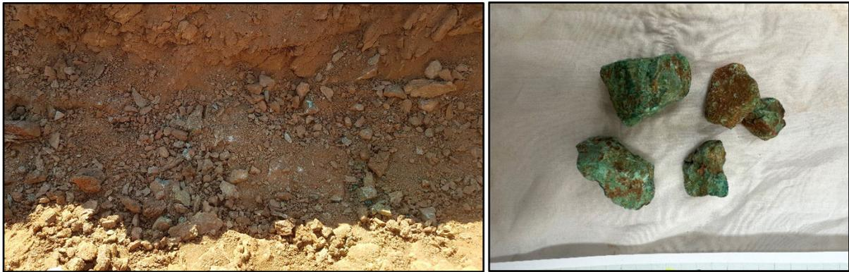
**Photo 2:** Copper-oxide (malachite) mineralisation in surface excavation and malachite rich rock chips at Browns prospect
