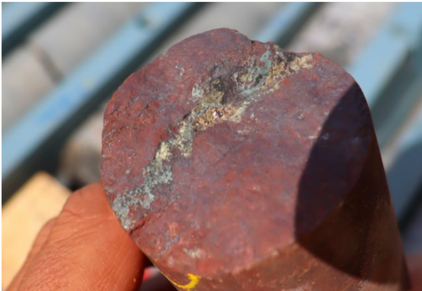
Figure 9 Sulphide vein with chalcocite, bornite and native copper, taken from hole DD21EBD0003W2, approx. 615m. This vein is located in the haematite cap overlying the Hiltaba suite granite sill which has typically not been enriched in Cu in other holes.
