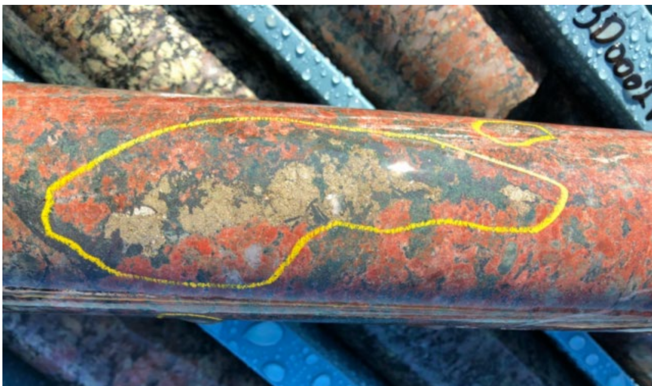
Figure 8 Sulphide blebs and intense “red rock” (K Feldspar + accessory haematite) alteration in hole DD21EBD0002W1. This material was encountered in Donington Suite granite at significant depth (1,241m). Strong red rock alteration, plus biotite and sericite, was typical of the granite in this hole, but atypical of Donington Suite Granite encountered in other holes, suggesting potential proximity to a hydrothermally significant structure. Portable XRF has confirmed elevated copper values in the sulphide, validating the field identification of chalcopyrite.
