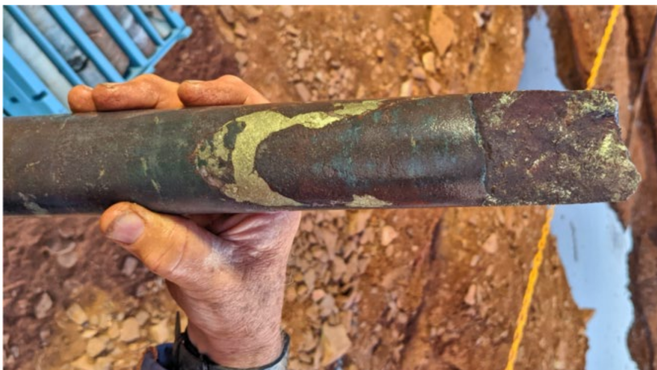
Figure 7 Massive chalcopyrite vein within a broader mineralised envelope of approximately 24.m consisting of blebs and veinlets of similar sulphides in an intensely haematised metasedimentary host rock, DD21EBD0002W1.
