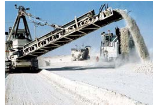
Wirtgen Surface Miner Cutting Salt
