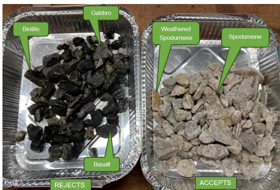
Figure 9. Typical composition of ore sorted Rejects and Accepts.
