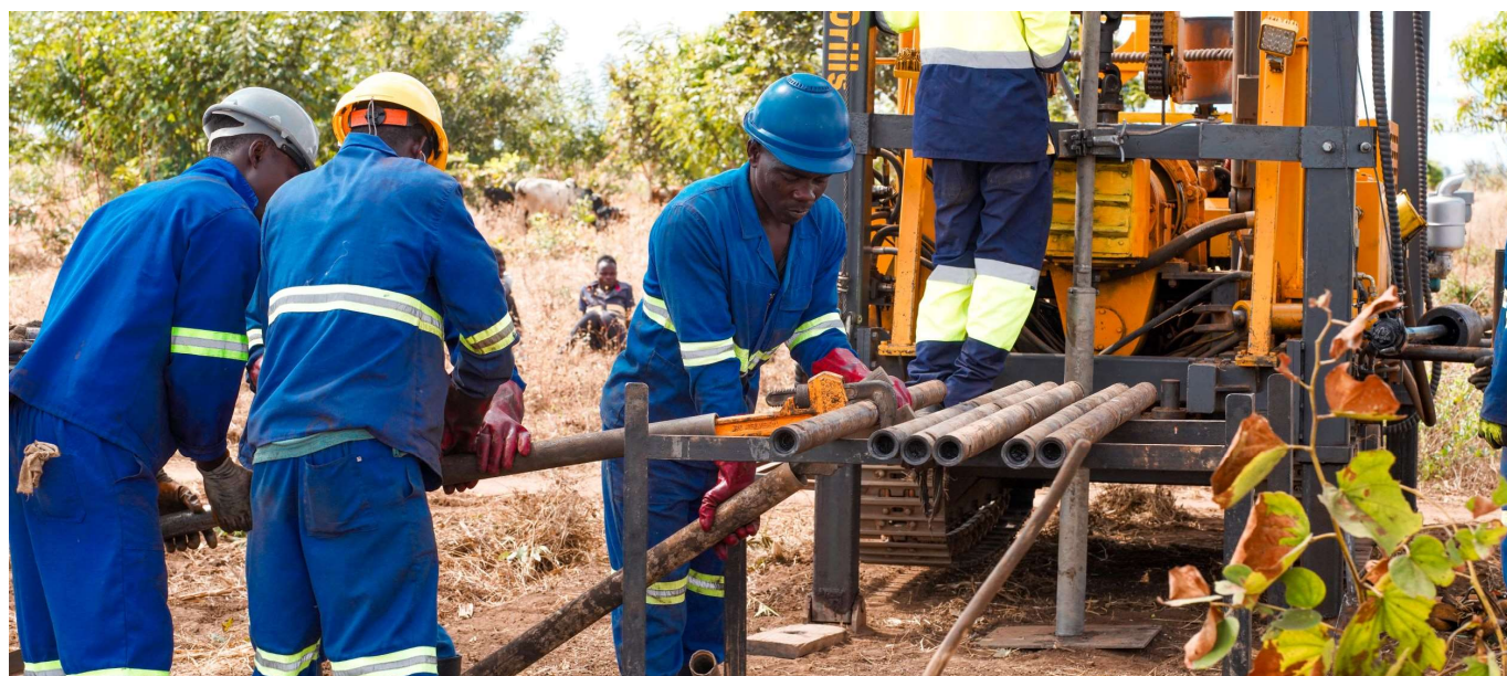
Figure 5: Core drilling at Kasiya
