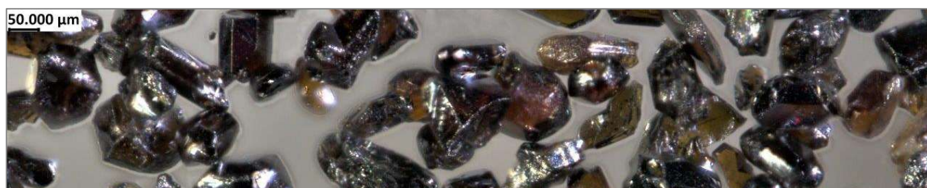
Figure 6: Photomicrograph of high purity rutile product 97.2% TiO 2
