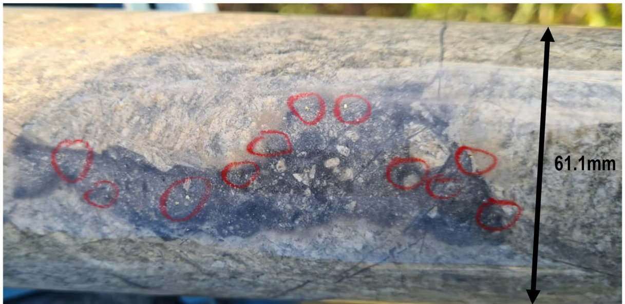
Photo 3. Visible Gold (circled red) in hole 25ENDD001 at 173.5m down hole in quartz veins within granite host rock. Drill core diameter is 61.1mm.
