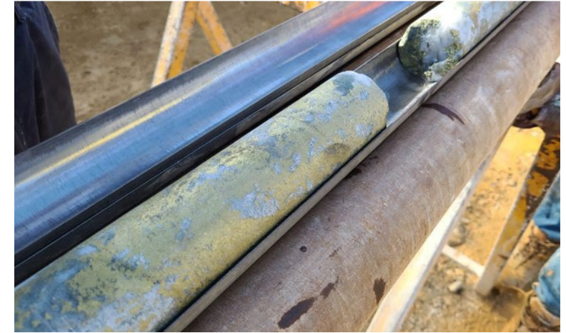
Visible Chalcopyrite Stringer Veins from Near Mine Exploration (MCDD015).
