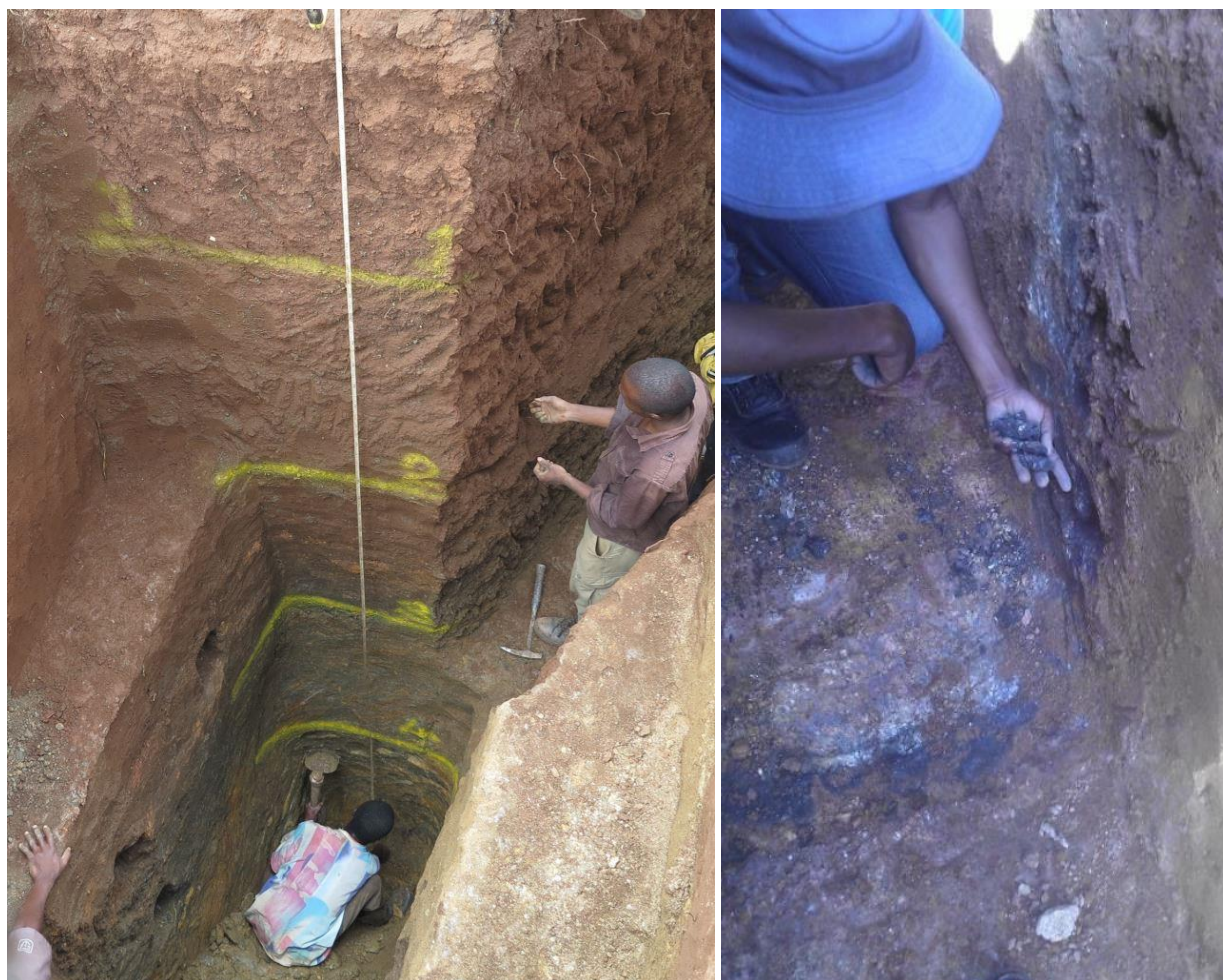
Figure 5 (Left). First pit excavated at Dedza Mountain West (DMW) Prospect showing flake graphite hosted within very soft saprolite to 5m depth. Figure 6 (Right). High-grade flake graphite hosted in saprolite exposed in trench at Dedza Mountain East (DME) Prospect.
