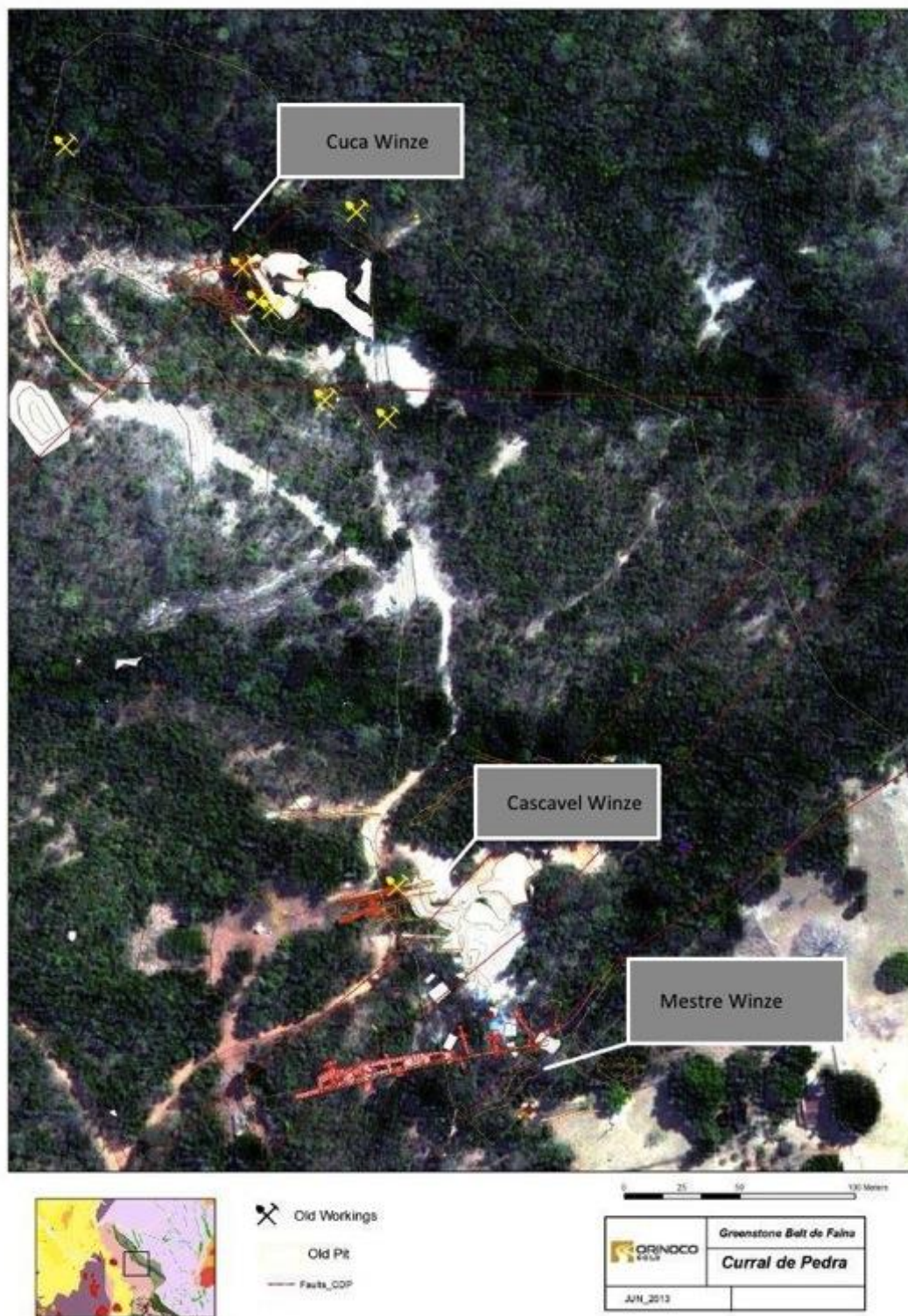
Figure 7 – Plan view of the location of all the artisanal workings identified to date, with the three winzes that have been bulk sampled highlighted.
