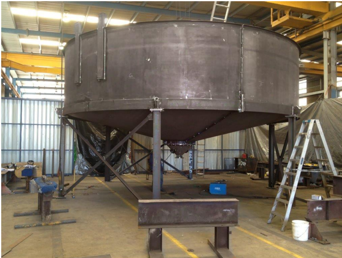
Figure 2 | Construction of 8 metre thickener for Riley Mine
