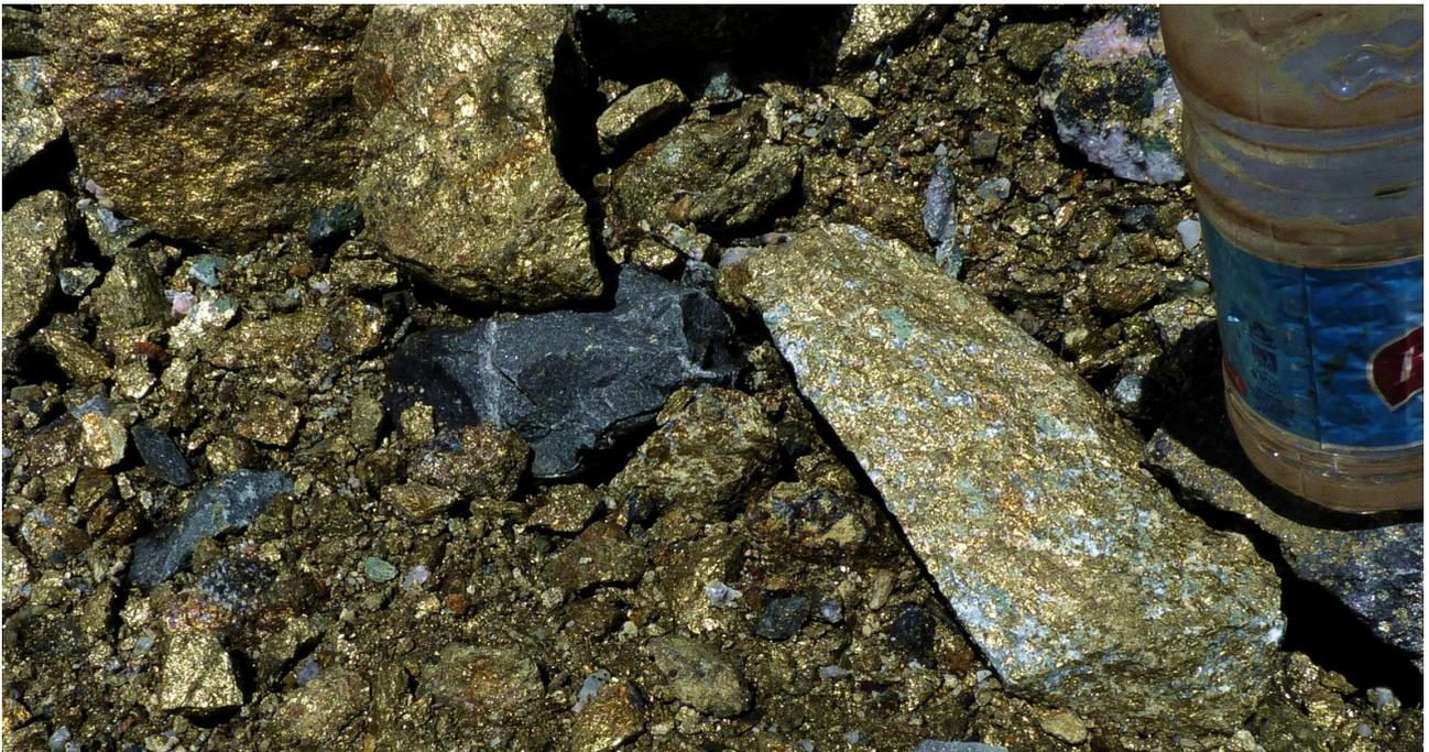
Figure 3: Massive primary copper ore chalcopyrite (yellow - chalcopyrite contains 34.6% copper), and bornite (63.3% copper) at just 12m from surface in the LM1-E pit, at grades suitable to be shipped as high-grade Direct Shipping Ore (DSO).
