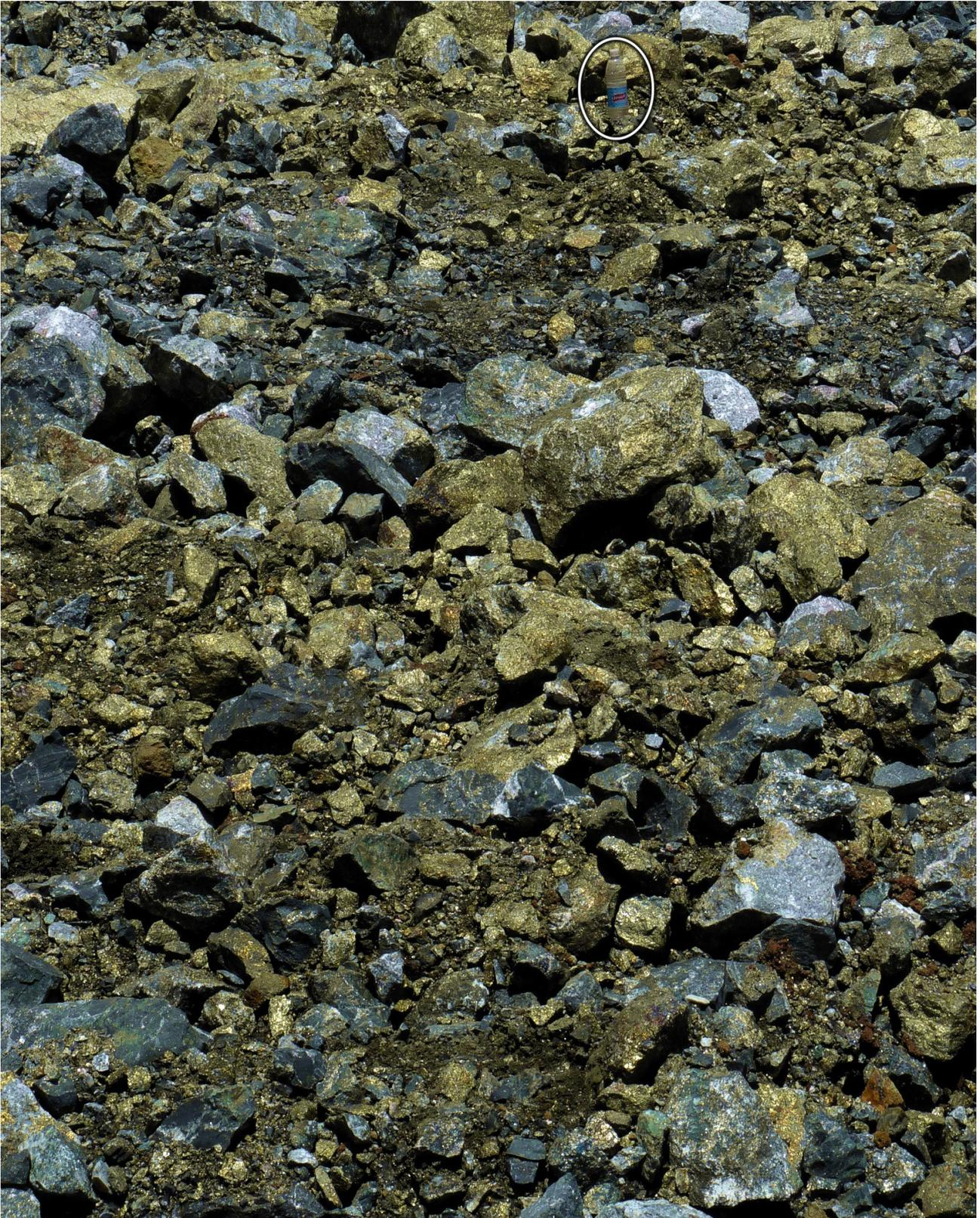
Figure 2: Massive primary copper ore chalcopyrite (yellow - chalcopyrite contains 34.6% copper), and bornite (63.3% copper) at just 12m from surface in the LM1-E pit, at grades suitable to be shipped as high-grade Direct Shipping Ore (DSO).
