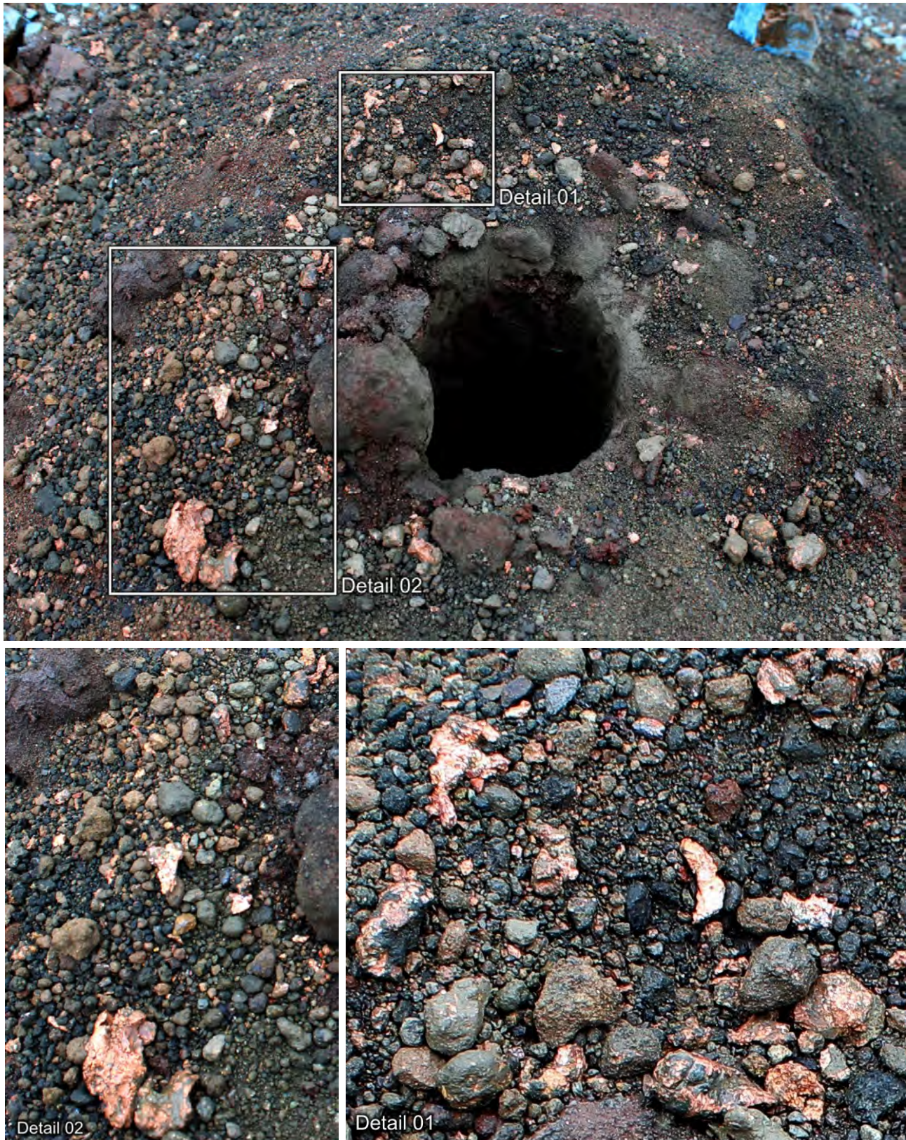
Figure 04: Example of open hole blast-hole drilling of completely dry sample, in high-grade native copper zones at LM, visually estimated at 20% Cu in this hole.
