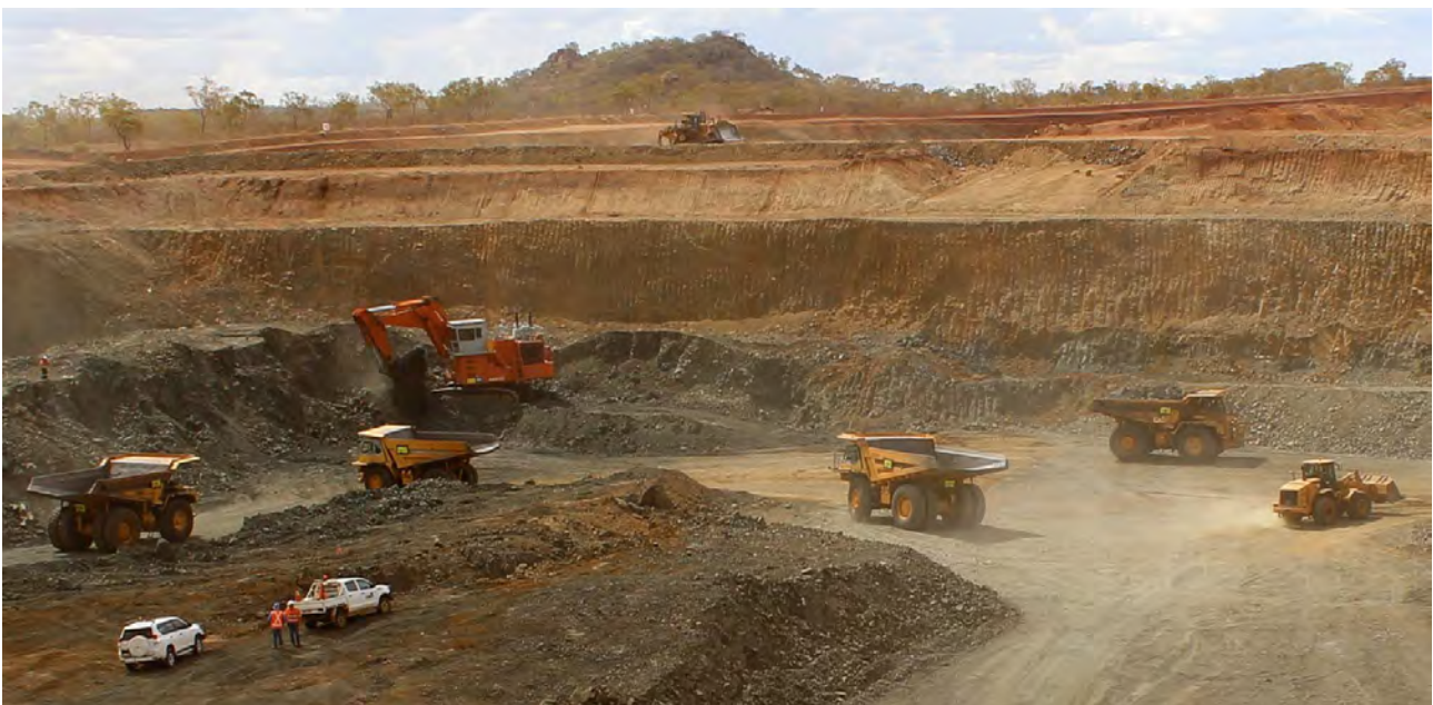
Figure 21: Las Minerale Stage-1 (LM1) Pit - with two diggers in ore working hard to keep ahead of a never ending procession of dump trucks transporting ore to the stockpiles.
