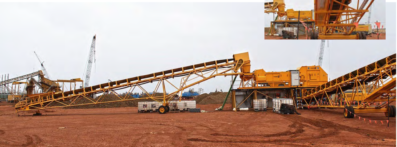
Figure 10: Ore Sorter assembled and ready for trial processing of ore towards the end of 2013.
