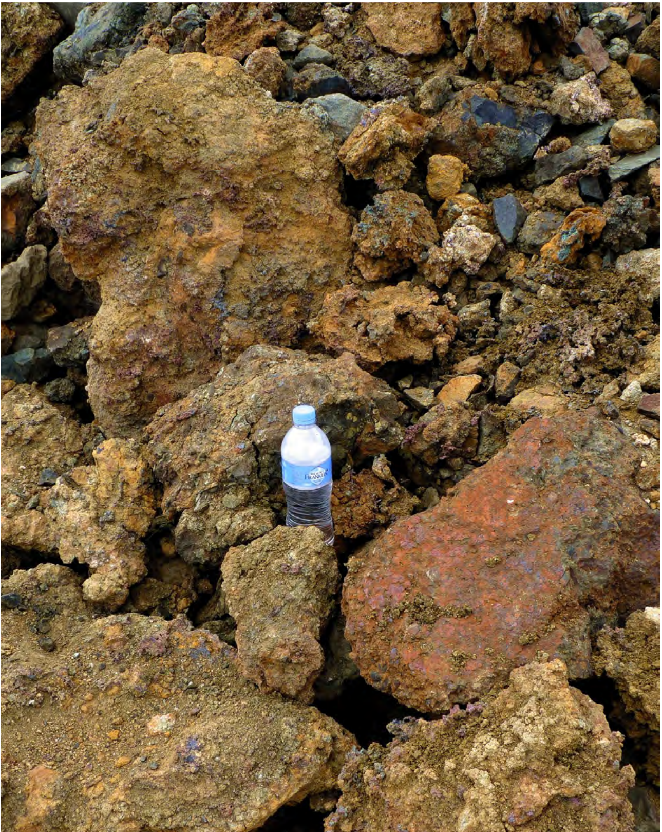
Figure 24: Example of high-grade coarse native copper stockpile on the ROM - see close-ups on following page.
