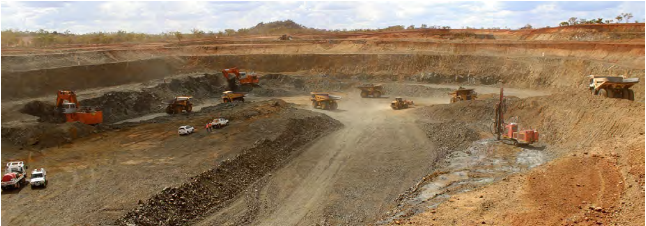
Figure 1: Las Minerale Stage-1 (LM1) Pit - with two diggers in ore working hard to keep ahead of a never ending procession of dump trucks transporting ore to the stockpiles.
