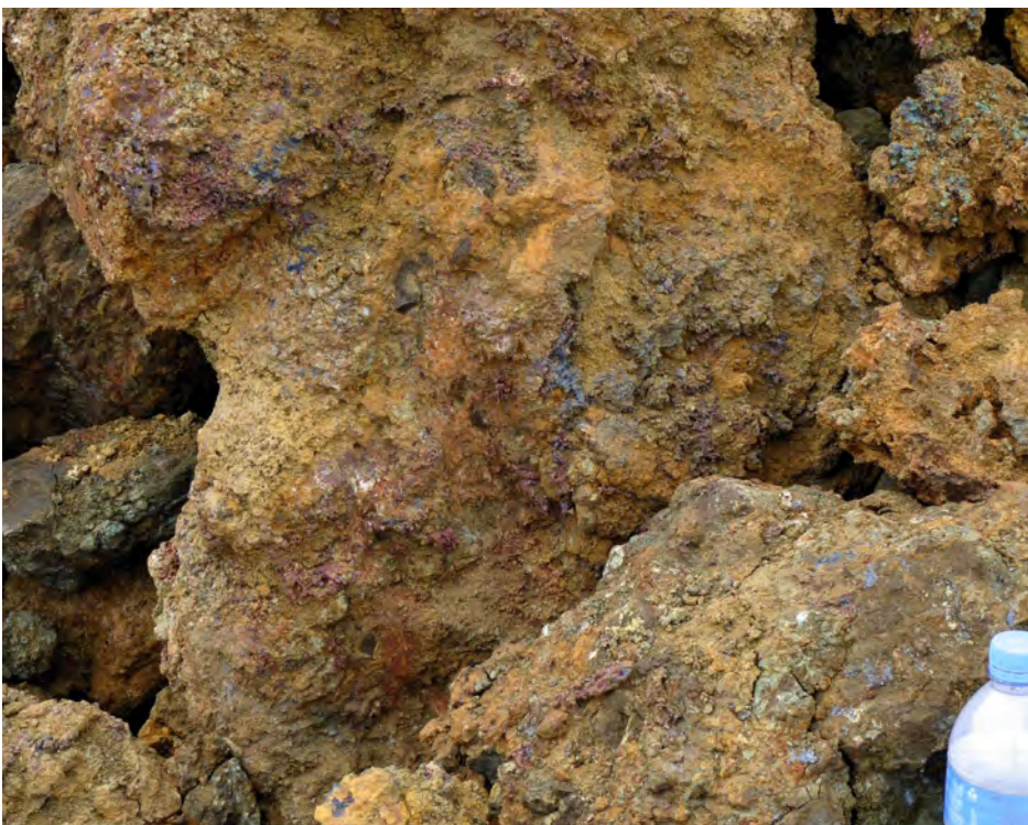
Figure 25: Details of previous page - example of high-grade native copper stockpile on the ROM, with close-ups of the previous image showing coarse native copper both in rock matrix and soft friable rock and clays.
