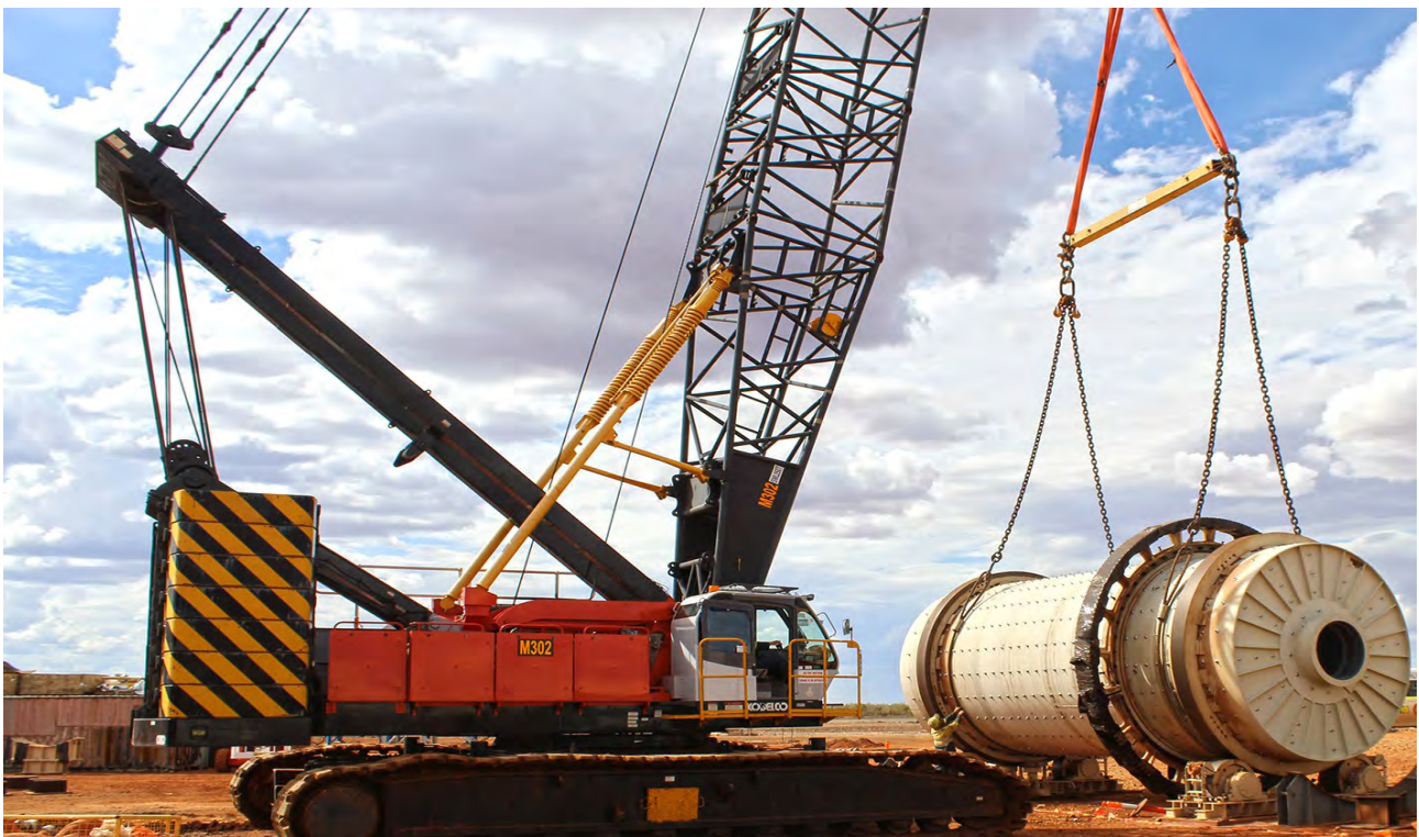
Figure 17: Gravity Thickener pumps and Walz crawler-crane moving De-agglomerator.
