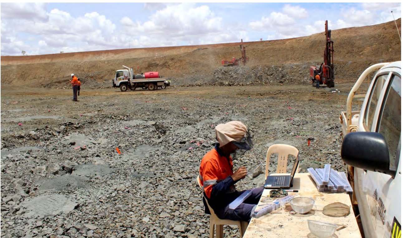
Figure 02 & 03: Blast-hole drilling and sampling at LM1 (LM Stage 1 starter pit)
