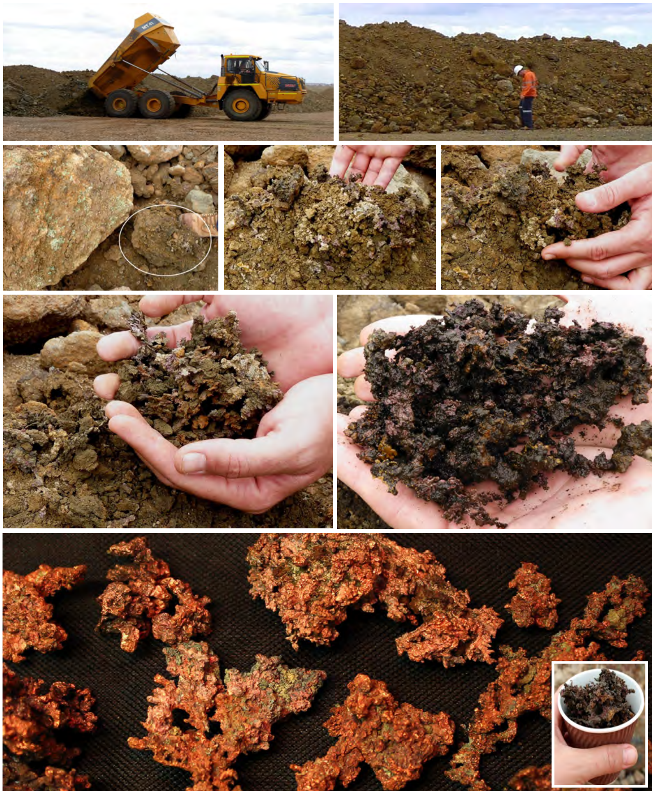
Figure 23: Example of high-grade native copper ore in soft friable matrix (dry green clays) straight from the pit. In sequential order, approximately 1 pound of copper nuggets are easily extracted by hand then cleaned with water to remove the soft, friable gangue material, leaving a near pure copper metal product with little effort. Bottom image; close-up of the copper nuggets after being cleaned with a dish-washing brush and water to reveal the copper metal and inset; a pound of copper currently costs less than a cup of coffee, a scenario the Company believes will change dramatically in favour of copper in the years ahead.
