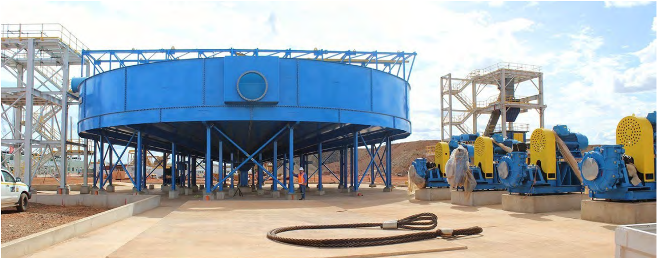
Figure 18: Gravity Thickener & pumps
