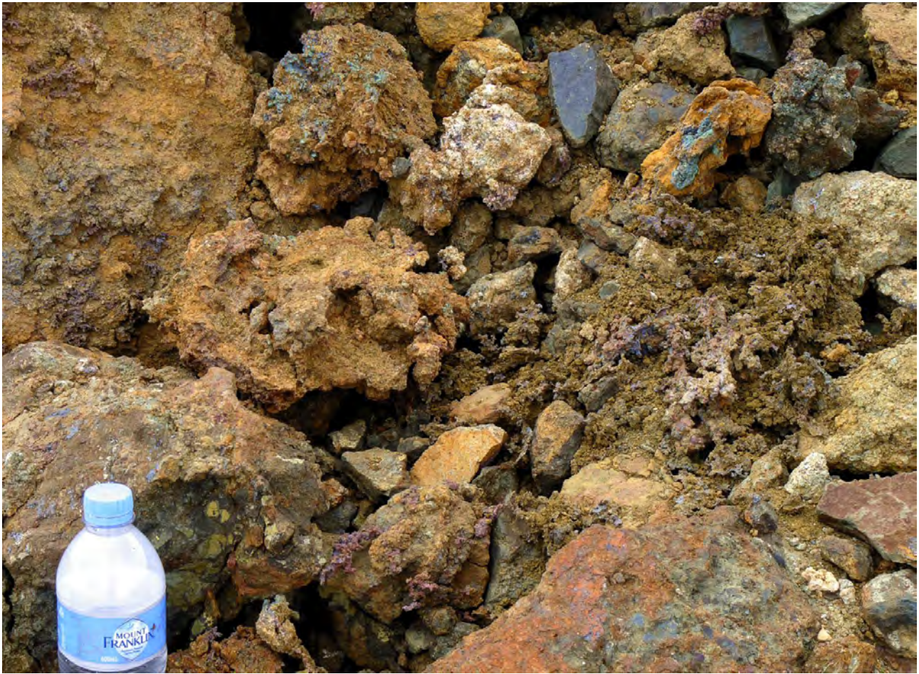
Figure 25: Details of previous page - example of high-grade native copper stockpile on the ROM, with close-ups of the previous image showing coarse native copper both in rock matrix and soft friable rock and clays.
