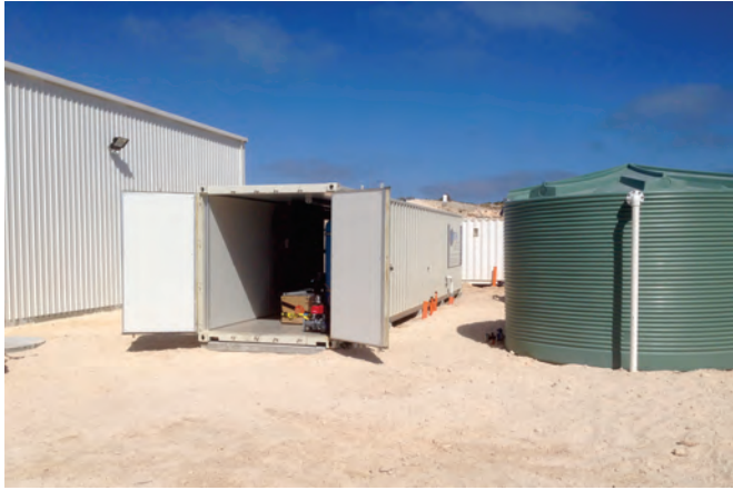
Containerised desalination pilot plant delivered to Garden Island (L), interior of desalination pilot plant (R)
