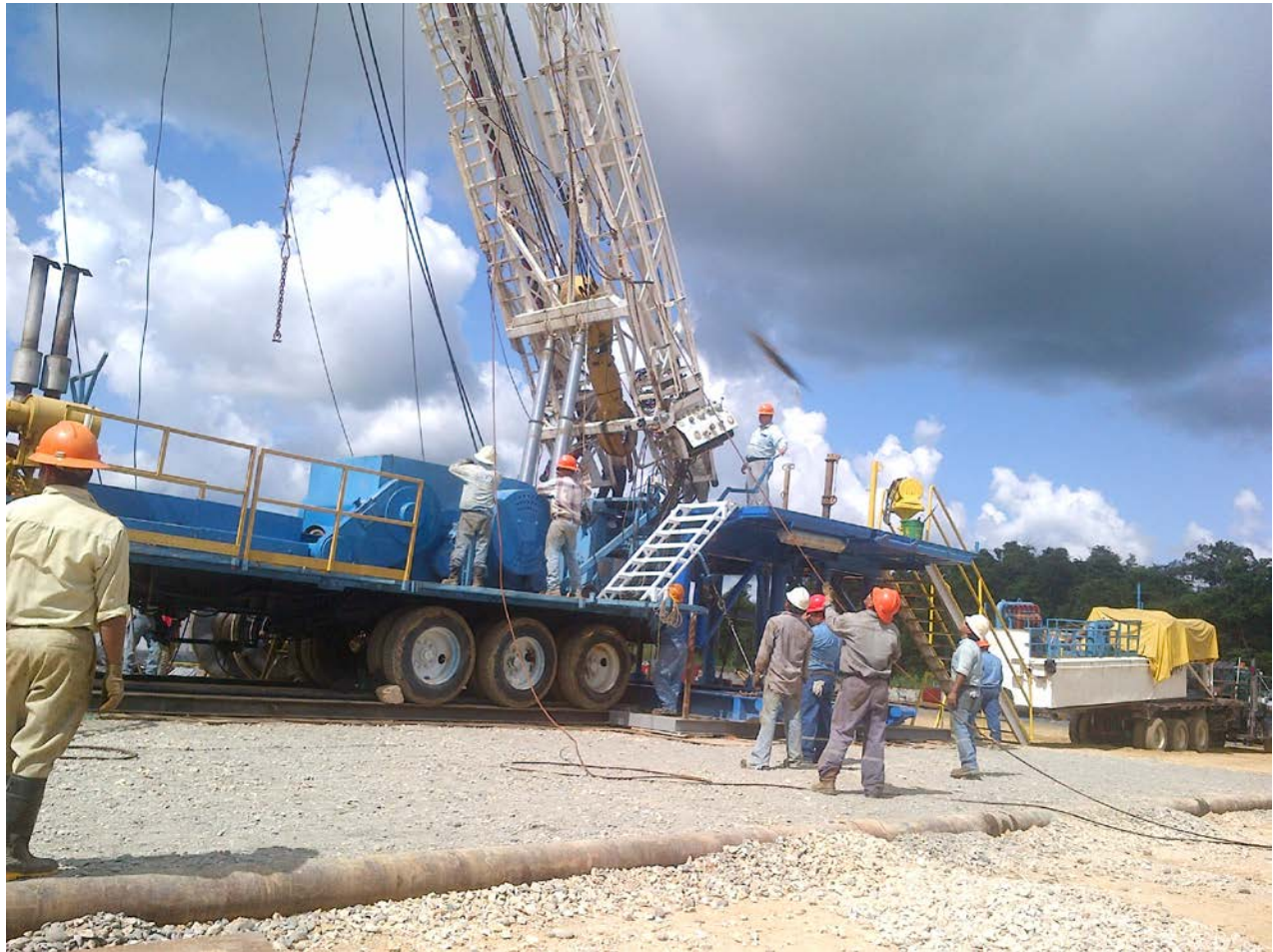
Rigging up mast on Atzam #5 location
