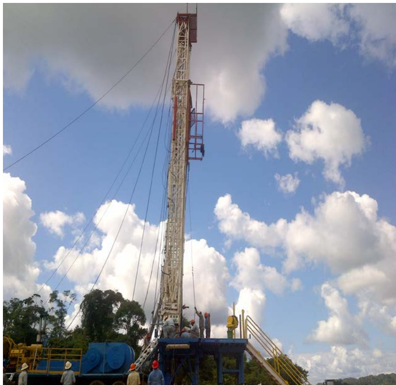
Atzam #5 Drill Site- Setting the drill mast on the Harold Lee 500 rig
