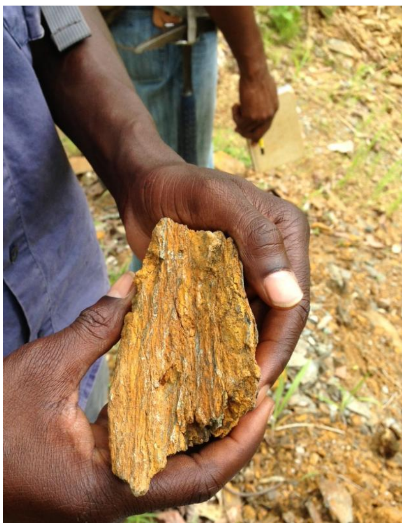
Figure 5 – Strongly carbonate altered schist in workings south of Antenna. Grab samples here returned 14.5g/t Au from quartz, and 4.68g/t from schist.
