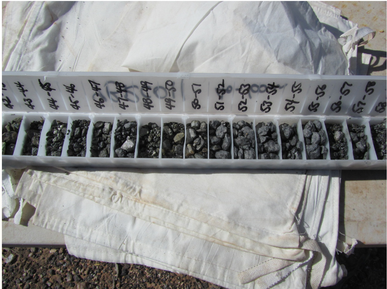
Figure 6. High-grade graphite RC Chips from hole YBRC011 45-59m – 14m @ 21.5% TGC
