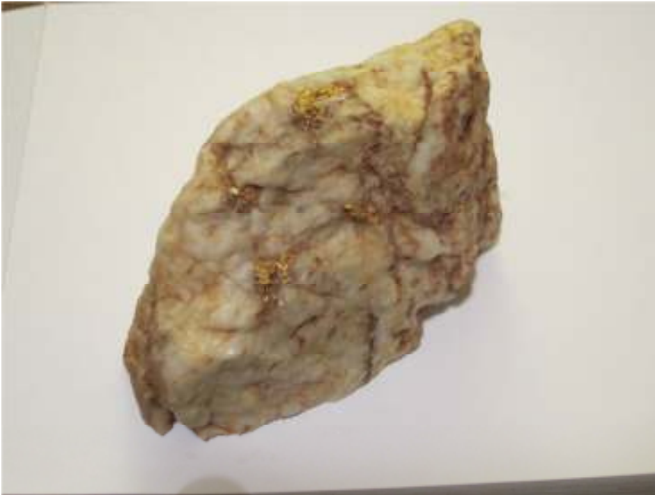
Figure 5: Visible coarse gold in quartz veins at the White Quartz Hill gold prospect
