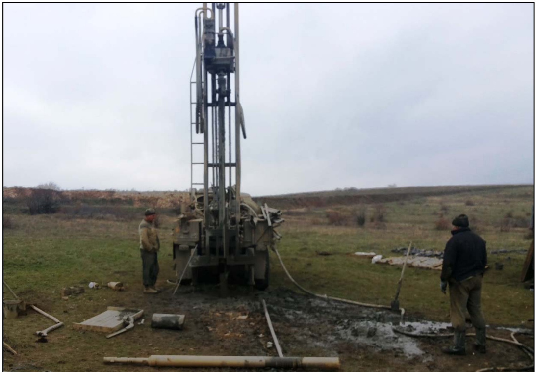
Figure 1 Drilling at gold and silver Bobrikovo project, large diameter coring bit in the foreground
