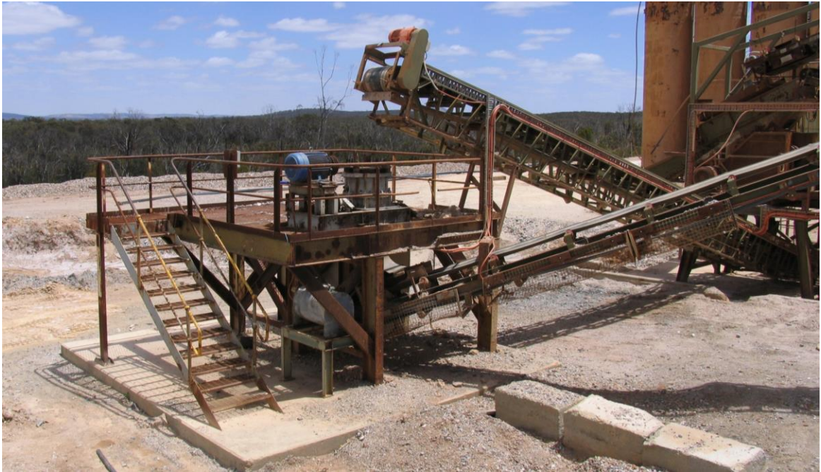
Fiddlers Creek Cone Crusher installed at Inglewood
