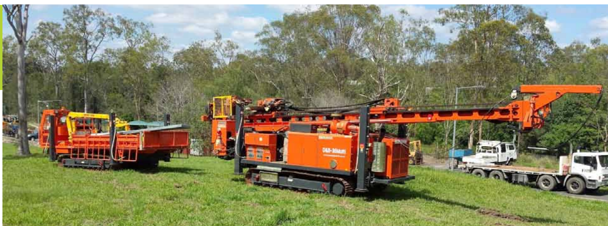
Image above: A track mounted drilling rig that is well suited for the tropical vegetation and steep terrain
