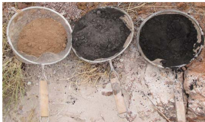
Figure 3: RC sample pulps showing comparison of grey and graphitic altered, with adjacent unaltered Gardiner Sandstone.
