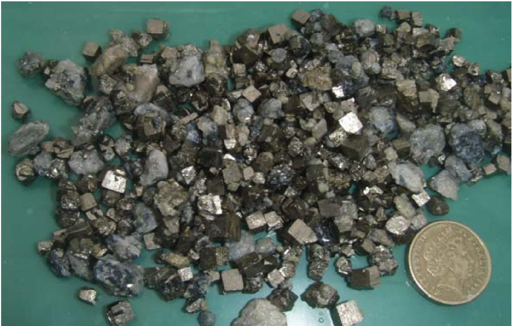
Martins Shaft: SGRRC0003, cubic arsenopyrite, 42-43m, 4.21g/t Au.
