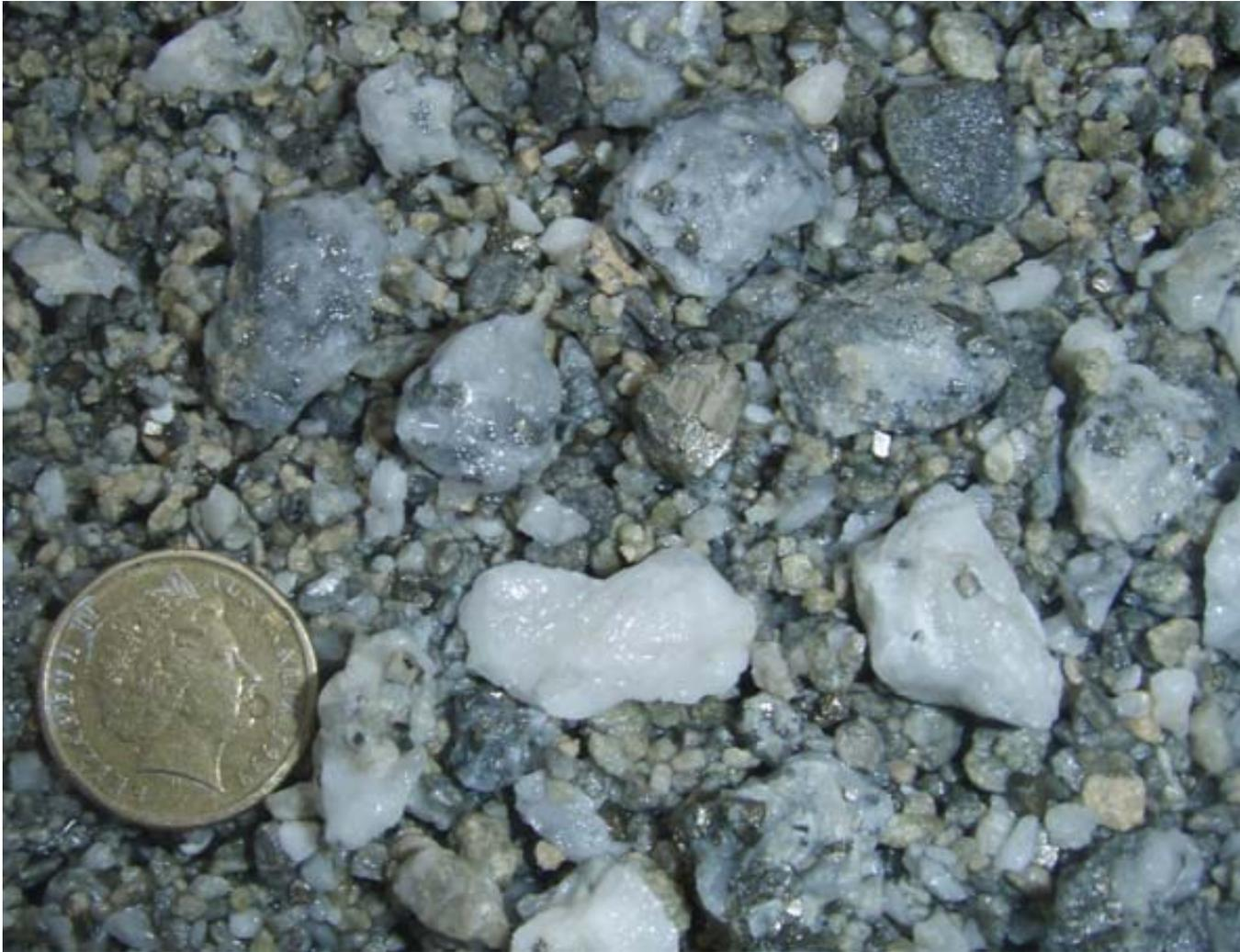
Martins Shaft. SGRRC0011, euhedral pyrite, 60m-61m. 1.53 grams per tonne Au.
