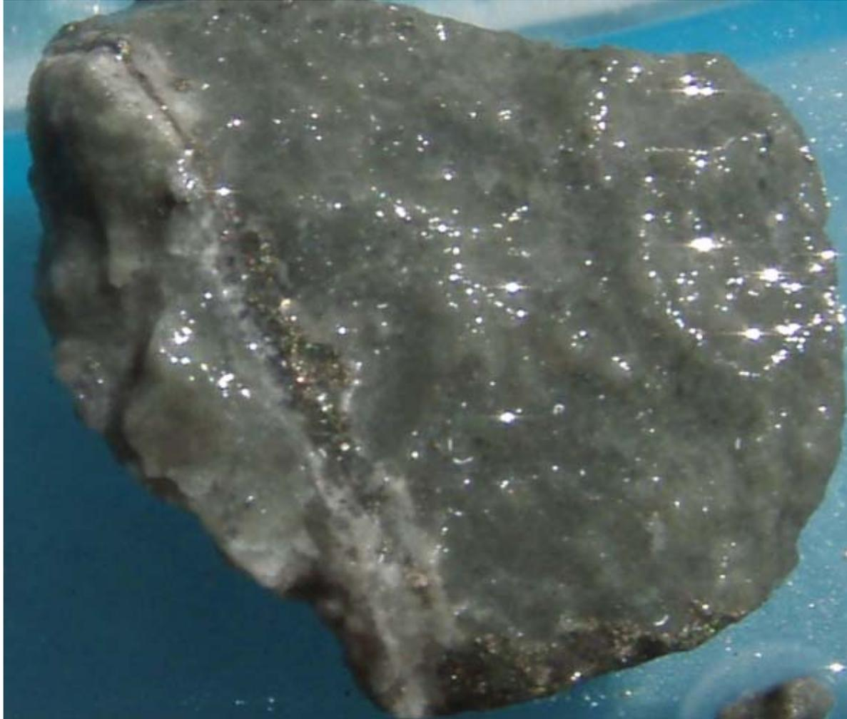
Martins Shaft. SGRRC0003, Sheeted vein alteration, 27m-28m, sulphide layer (2mm wide) and pale green quartz-sericite selvage.
