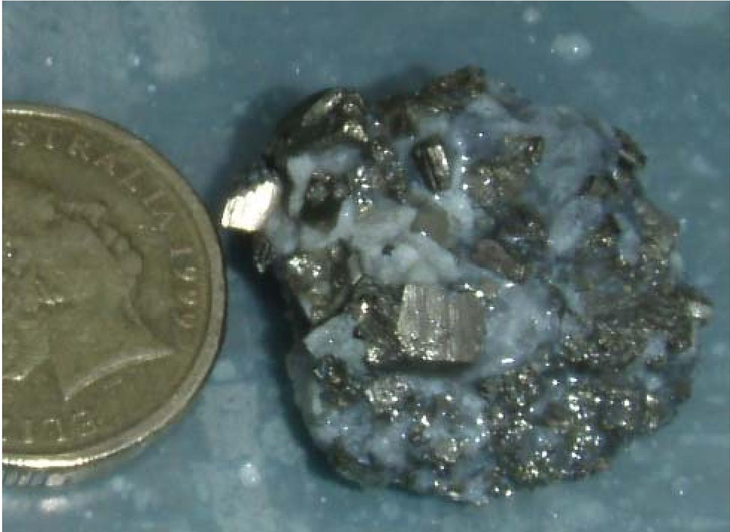
Martins Shaft, SGRRC017 euhedral pyrite and arsenopyrite, 86-87m,
