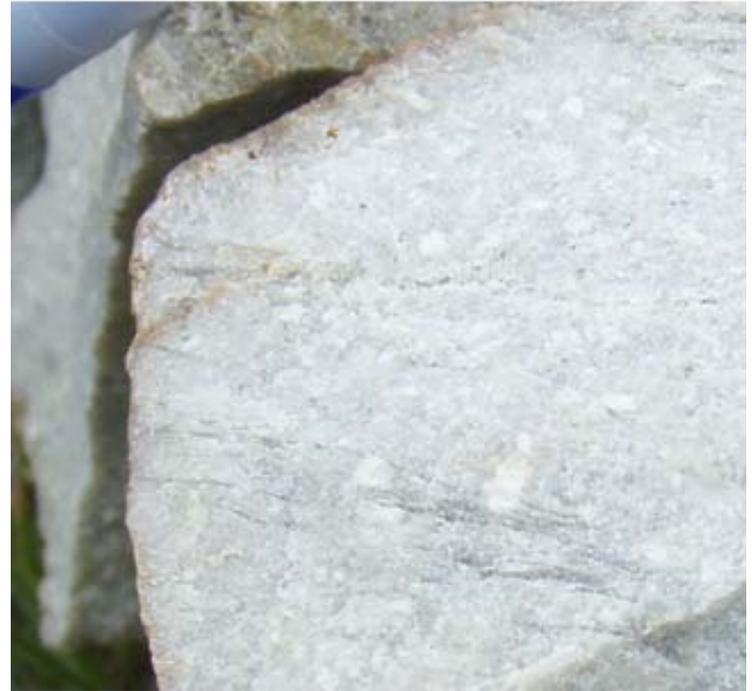
Martins Shaft, Gold-bearing Ore, euhedral pyrite and arsenopyrite in sericite-quartz (phyllic) altered felsic dyke.
