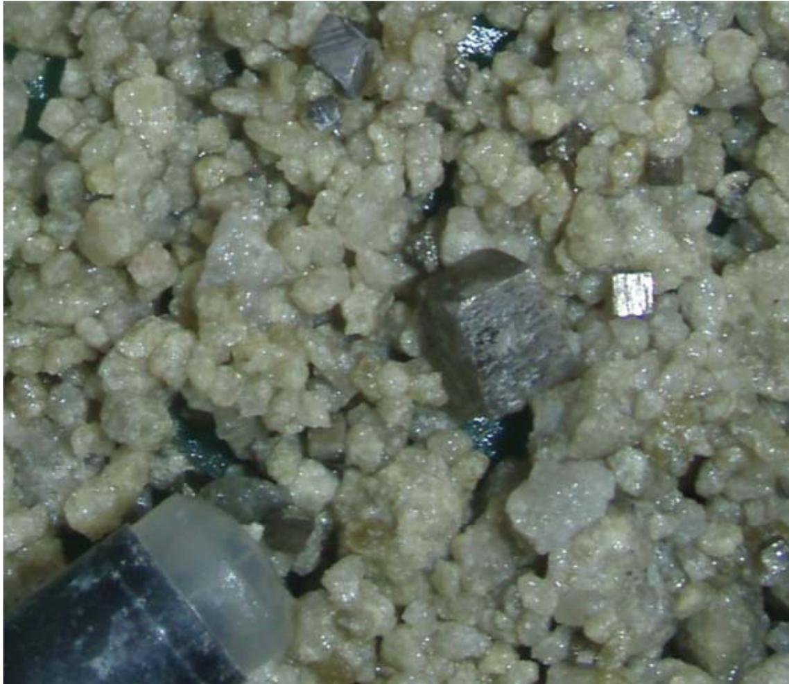
Martins Shaft. SGRR0011, euhedral pyrite and arsenopyrite in quartz, 60m-61m, 1.53 grams per tonne Au.
