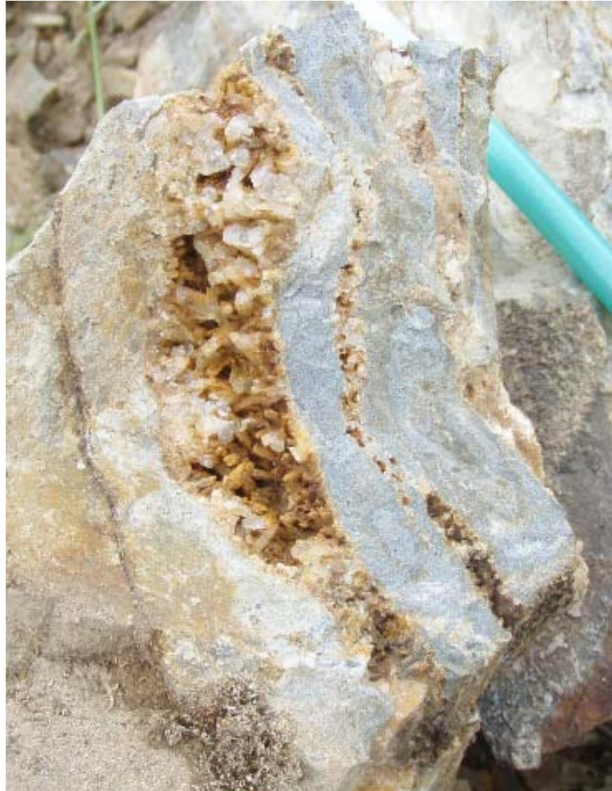
SGRRC0003, Sheeted vein with arsenopyrite and pyrite with white sericitic alteration selvage, vein 0.5-2mm wide, 53-54m down hole depth.
