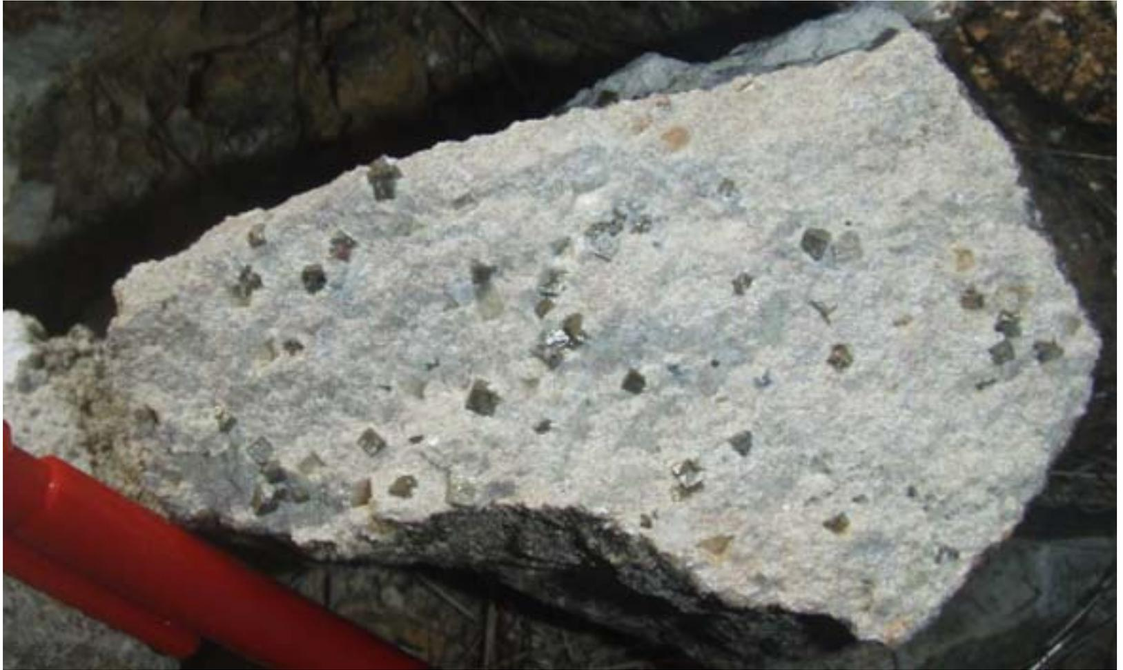
Hudsons McCrossins (HM7), late stage, porphyritic dyke with disseminated cubic pyrite and arsenopyrite. Phyllic alteration, assayed up to 1.87g/t Au.
