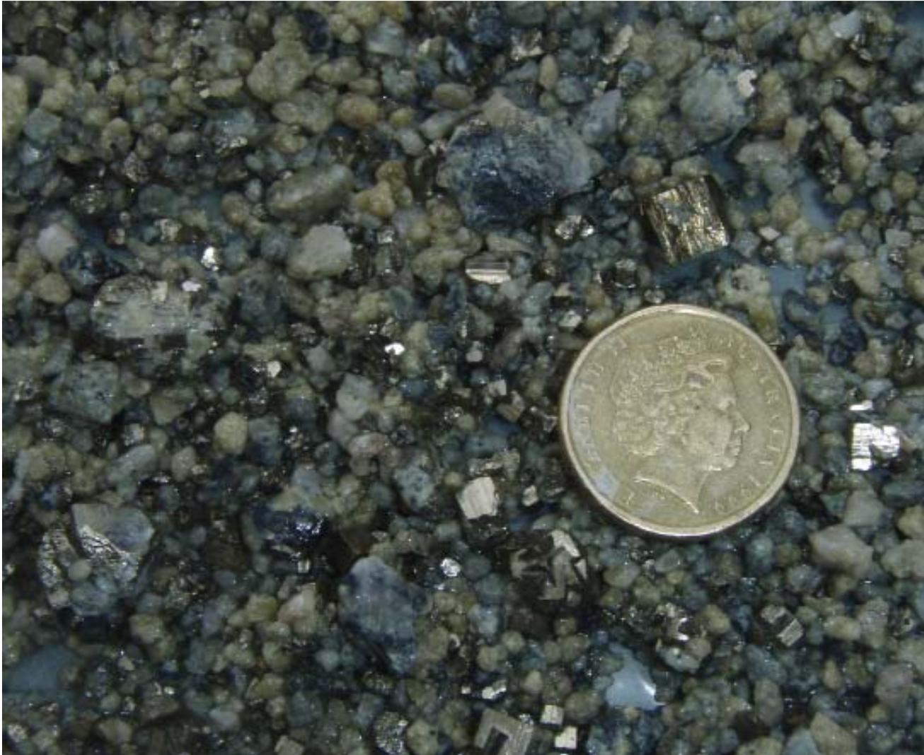
Martins Shaft, SGRRC017 euhedral pyrite and arsenopyrite, 86-89m.
