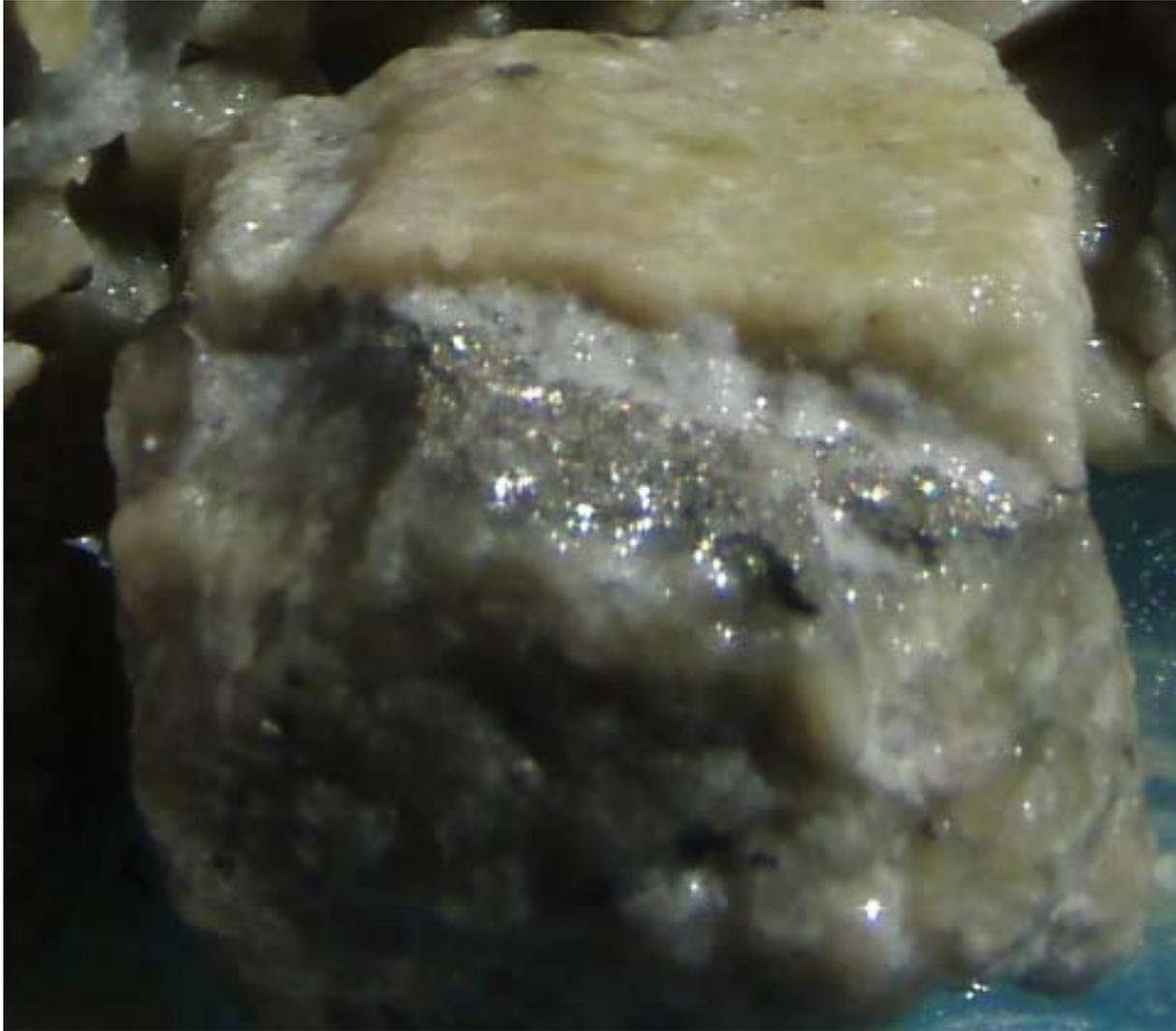
Martins Shaft. SGRRC0003, Surface of sheeted vein alteration, studded with 0.5mm wide arsenopyrite, 30m-31m.
