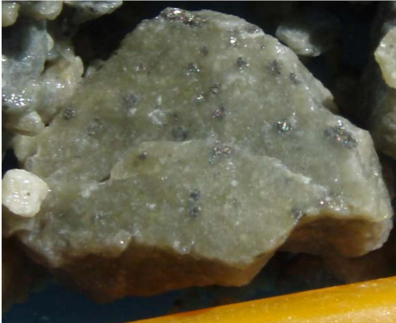
SGRRC011, Reduced IRGS phyllic alteration (green sericite, quartz and sulphides); pyrite cubes centre, rhombic arsenopyrite cubes to left of centre, 54-55m.
