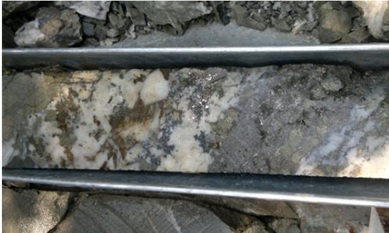
**Figure 3:** Memot – Anchor Prospect: visual logging identifies sulphide alteration.
