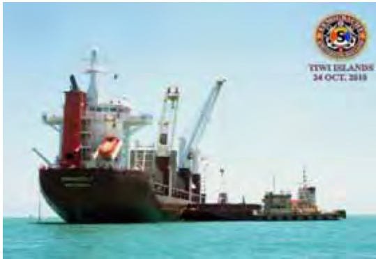
Loading from barge to ship via grabs
