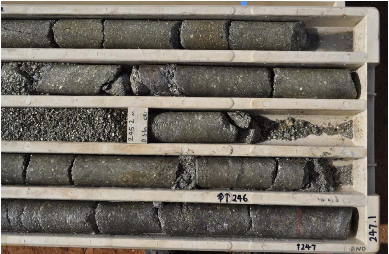
Photographs 1 and 2. – ML6750 “One Mile” - Diamond drill core from the two halves of Tray 9 from hole SPOM012 showing massive sulphides from this hole between 242.8m and 247.1m.
