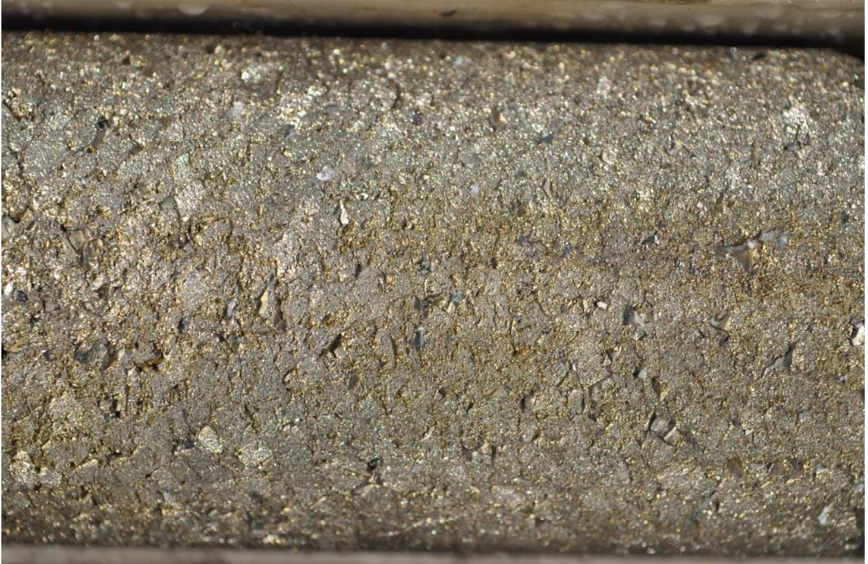
Photograph 3. – ML6750 “One Mile” – Close-up photograph of diamond drill core from hole SPOM012 showing massive sulphides. The coarse-grained sulphides are principally pyrite with some chalcopyrite and sphalerite. Core diameter is 47.6mm.
