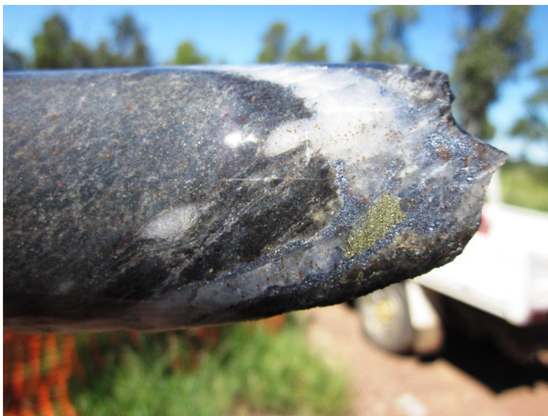
RCD69 at 260.85m: Quartz molybdenite (blue-grey colour) pyrite (yellow) vein in Anakie meta-sediment.
