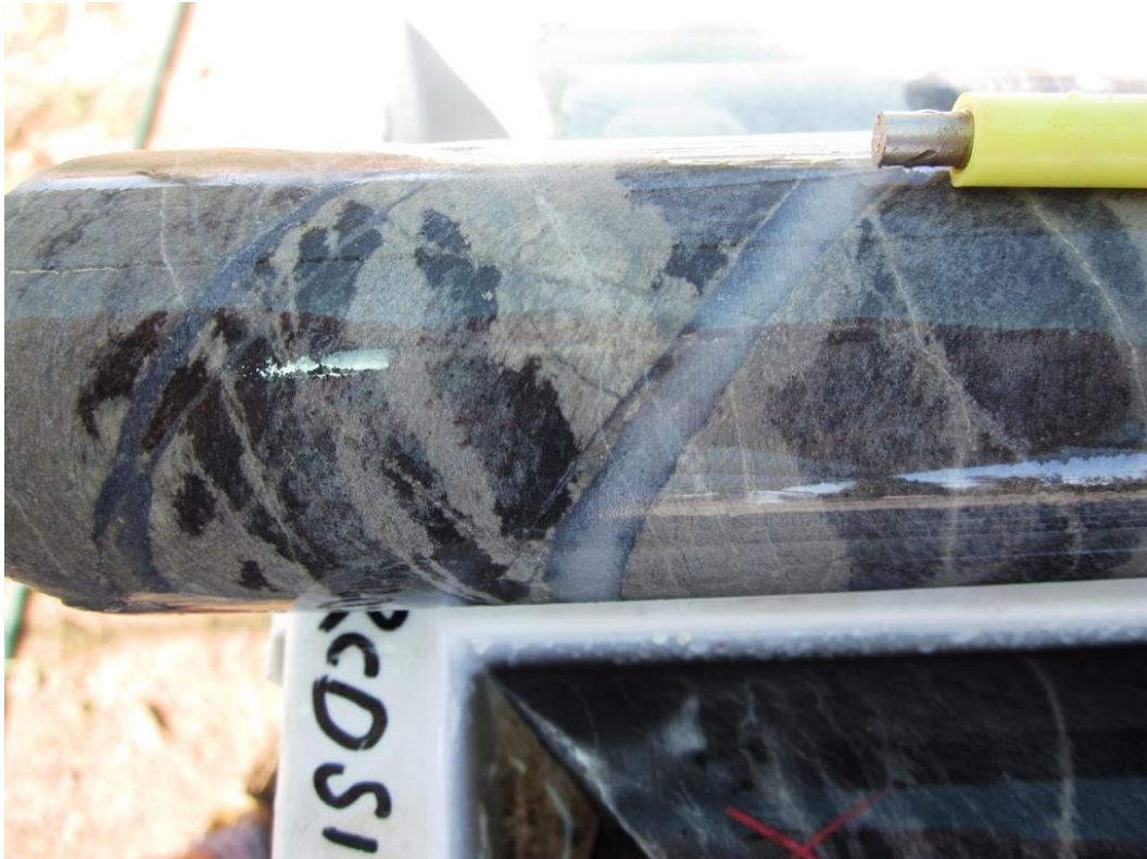
RCD69 at 360.5m: Parallel quartz molybdenite veins in strongly sericite altered Anakie metasediments
