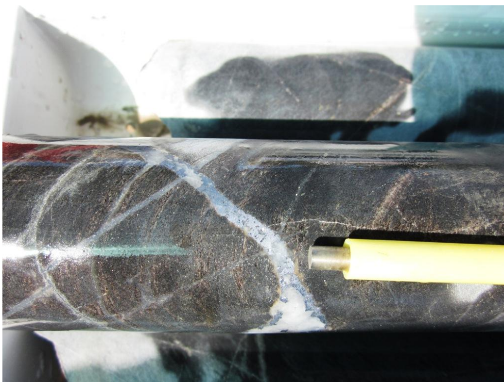
RCD69 at 320.1m: Coarse molybdenite (blue-grey) in quartz stockwork.
