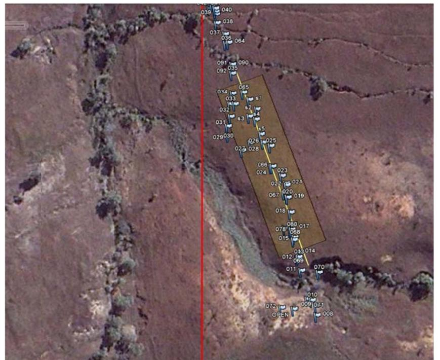
Figure 2: Artisanal shafts and trial mine pit location (yellow). Metallurgical test work sample collected in this area.
