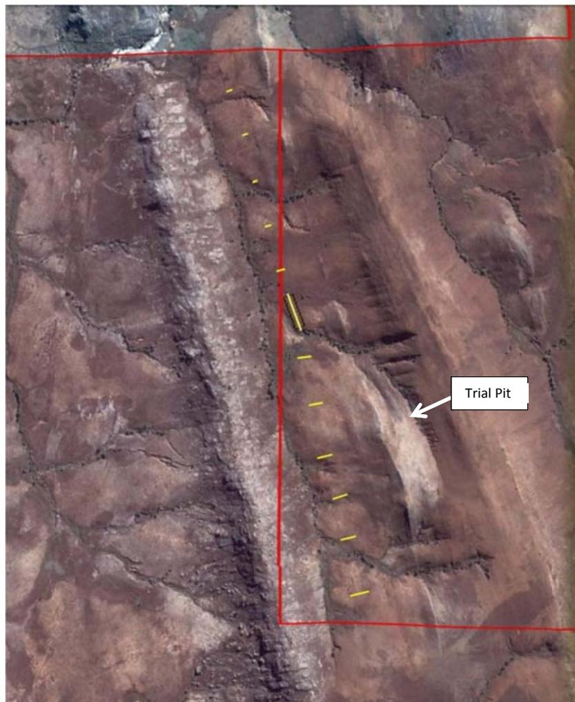
Figure 3: Schematic view of proposed 200m spaced costeans (yellow)
