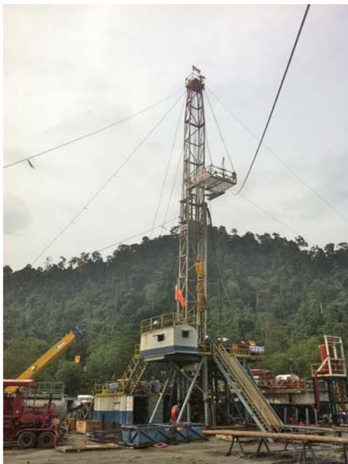
Pase A-2 achieved total depth ("TD") of 9,230 feet measured depth at 7:00 Jakarta time. All cement plugs have been cleaned out. One 4 1/2" EZSV packer has been drilled out, a final 4 1/2" EZSV packer has been pushed to well TD.
