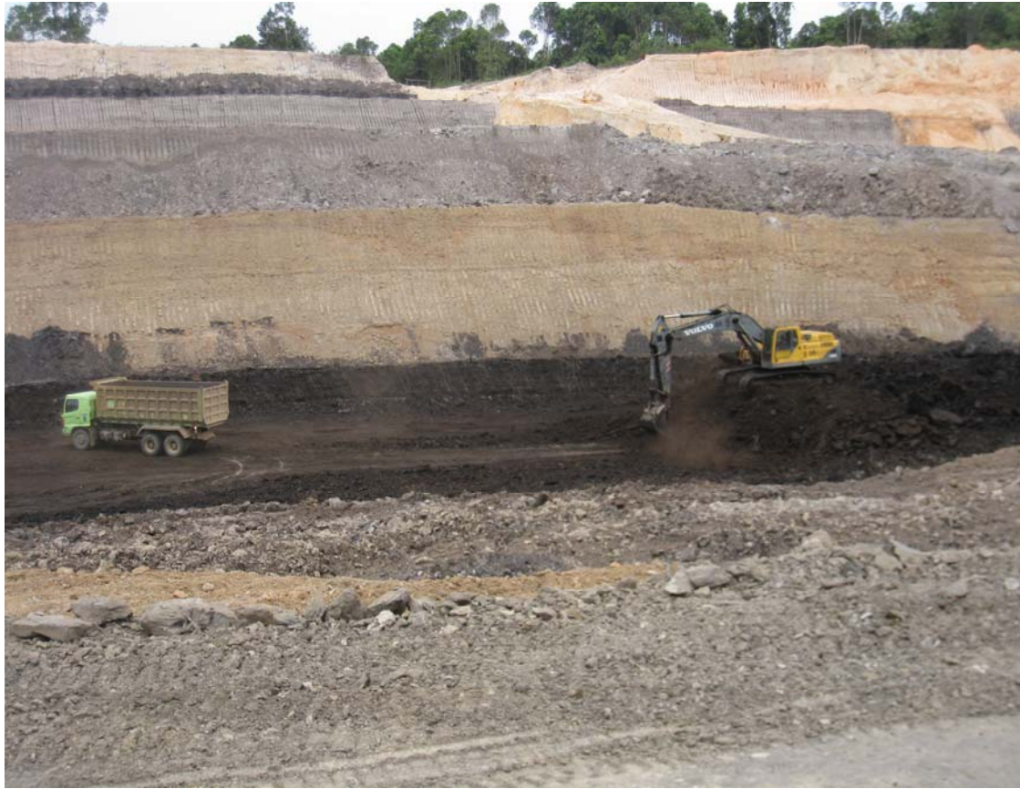
Plate 2: Photograph showing coal being extracted from the present mine pit bearing coal of minimum calorific value of 5100 Kcal/kg whilst stripping of overburden at another exposed coal seam is being carried out at the further end of the mine pit.
