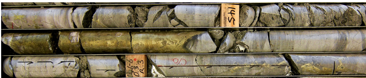
Figure 3: Massive sulphides intersected at approximately 146m in diamond drill hole DODH255.
