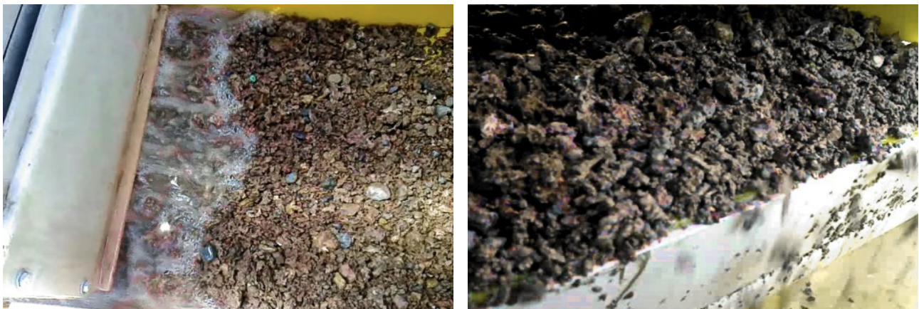
Figure 20: +4/-8mm native copper nuggets moving (left to right) through continuous alljig® screen, tipped into collector at right
