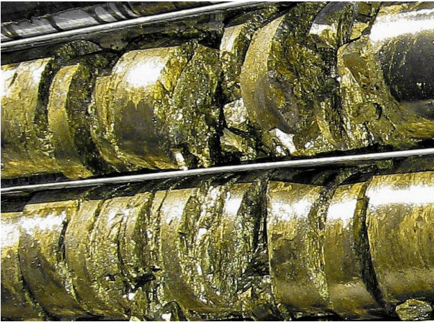
Figure 22: Primary copper ore (chalcopyrite contains 34.6% Cu) in diamond drill core LMDH013 (approx. 20-21m shown)
