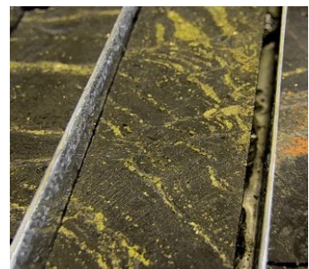
Figure 9: Primary ore (chalcocite = 34.6% Cu)
