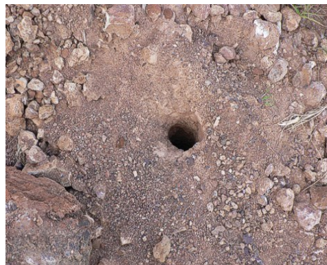
Figure 33: Example of typical bedrock hole. Using the Company's own RAB rig, the drill bit (hammer), pulverises rock into small chips, which are forced up to surface between the steel rod holding the hammer (string) and the outside of the open hole, under extreme air pressure. Material is collected from every metre, including the last metre which is drilled into hard bedrock, and bagged for logging and assay
