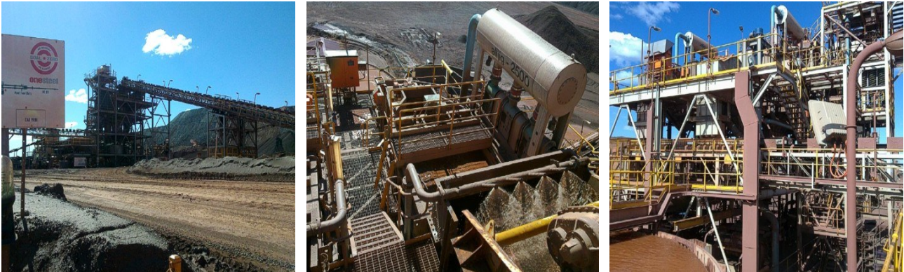
Figure 16: OneSteel's "Iron Duke" 3mtpa haematite concentrator, which uses "alljig®" gravity jigs to separate product from gangue material (waste), was visited by the metallurgy team in 2010. In spite of a density difference of just 1.3g/cm 3 , (product density 4.5g/cm 3 and waste density 3.2g/cm 3 ), successful gravity separation of product from waste is achieved at the rate of approximately 85%. At Rocklands, with a product density of 8.9g/cm 3 for native copper and approximately 3g/cm 3 for waste material, separation results are expected to be very high, as proven in this bulk test programme
