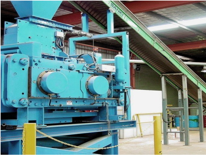
Figure 14: High Pressure Grinding Rolls (HPGR)
