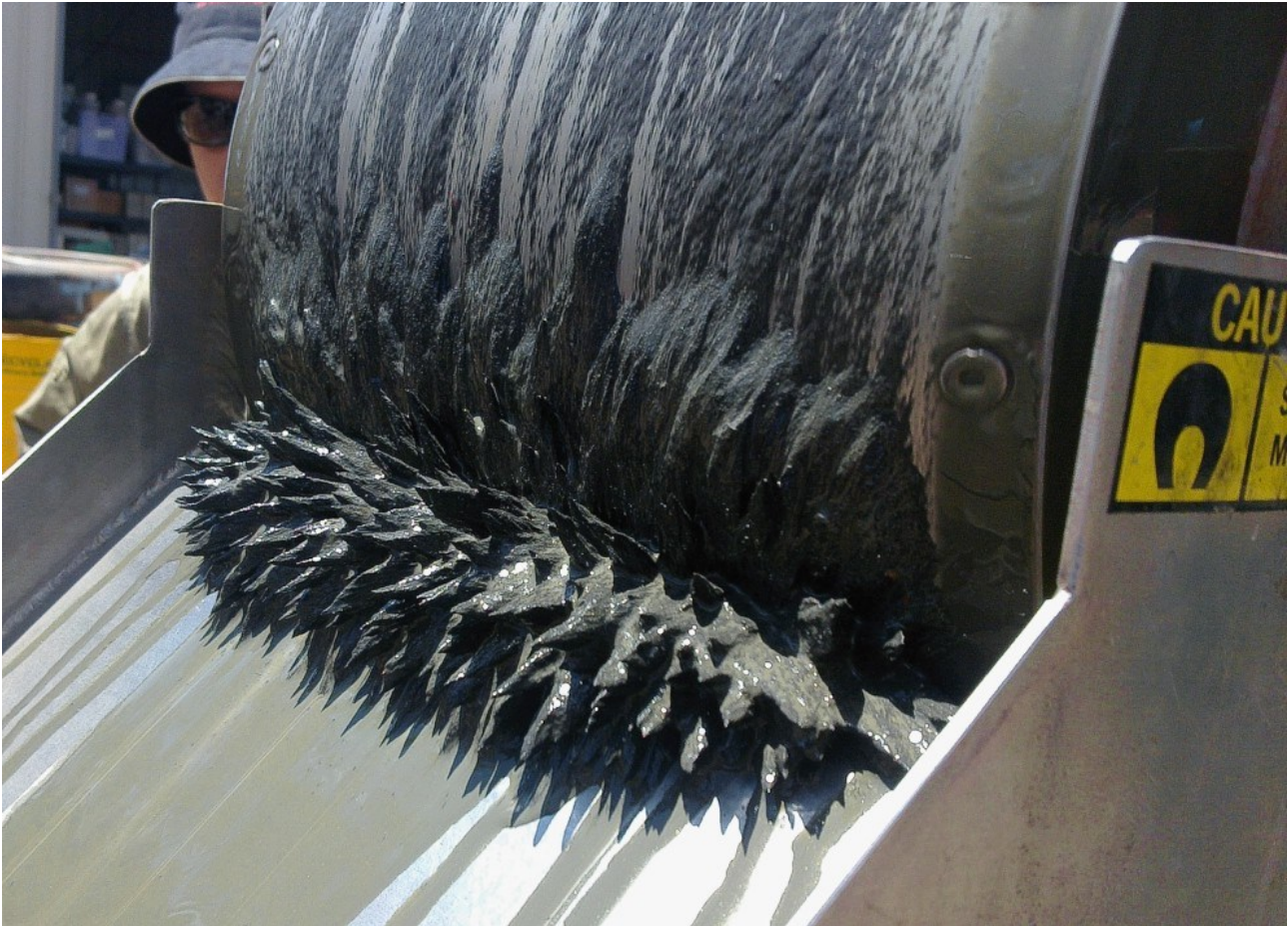
Figure 19: Removal of magnetite via Magnetic Separator
