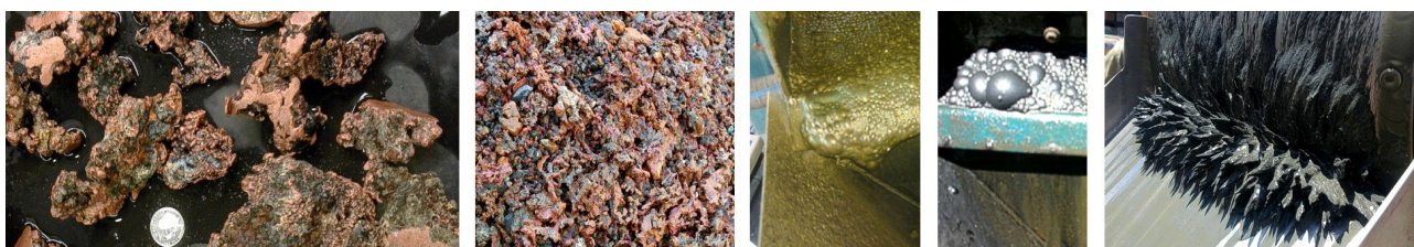
Figure 5: Various products from bulk-sample test-work (from left to right); large native copper nuggets (+40mm), smaller native copper nuggets (+4mm-40mm), flotation froth (primary circuit - chalcopyrite), flotation froth (primary circuit - chalcocite), magnetite separation.
