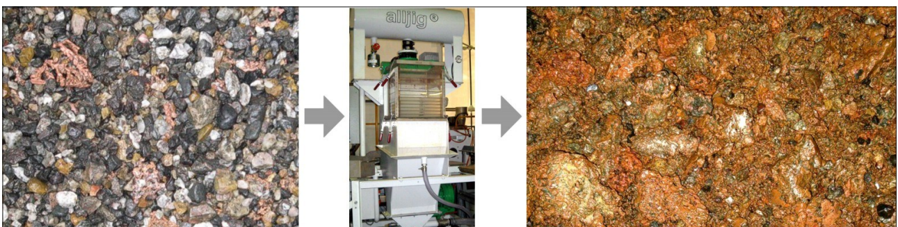
Figure 13: Product from Trommel (left), Static Test alljig® (centre) and +4mm Native Copper Concentrate Product (right)
