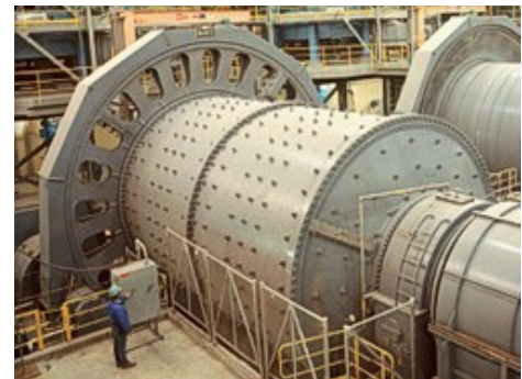
Figure 17: example of a ball mill, (Alcoa, Pt Henry), which grinds ore into fine powder, suitable for flotation
