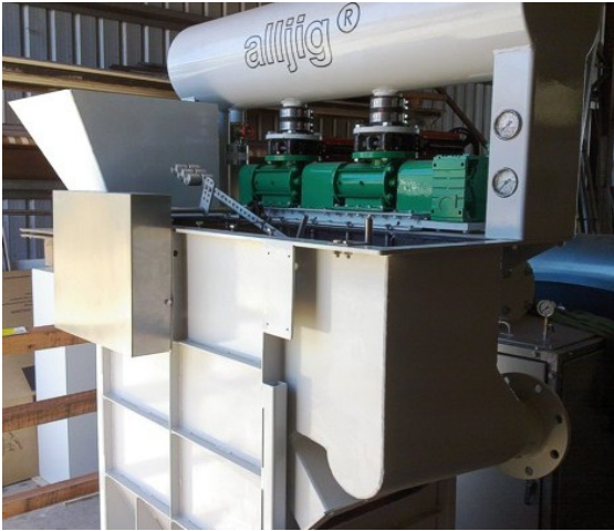
Figure 10: NAGROM Continuous Pilot 'alljig®'
