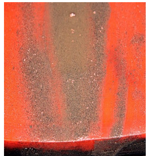
Figure 18: small amounts of residual native copper remaining after milling 10 tonnes of ore, indicating pre-treatment to remove the fine native copper prior to milling was successful
