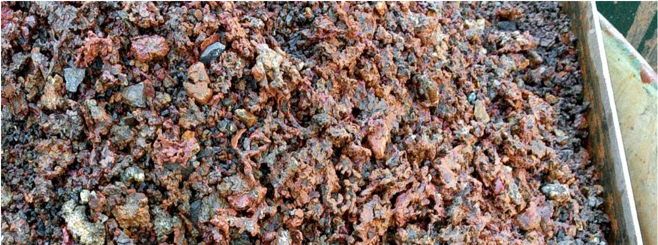
Figure 6: +4mm native copper nuggets (maximum size approximately 40mm), sitting in the collection tray after passing through the alljig® continuous jigging separation process
