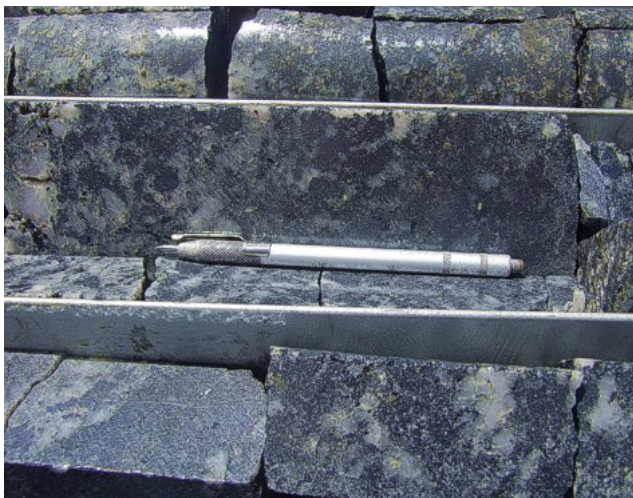
Figure 25: Copper ore (chalcocite), in diamond drill core DODH078 (blue-grey colour)
