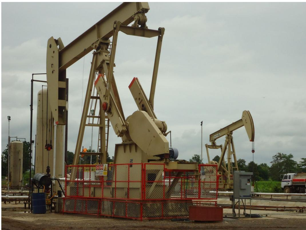
**Figure 5: Multiple production wells per location**
