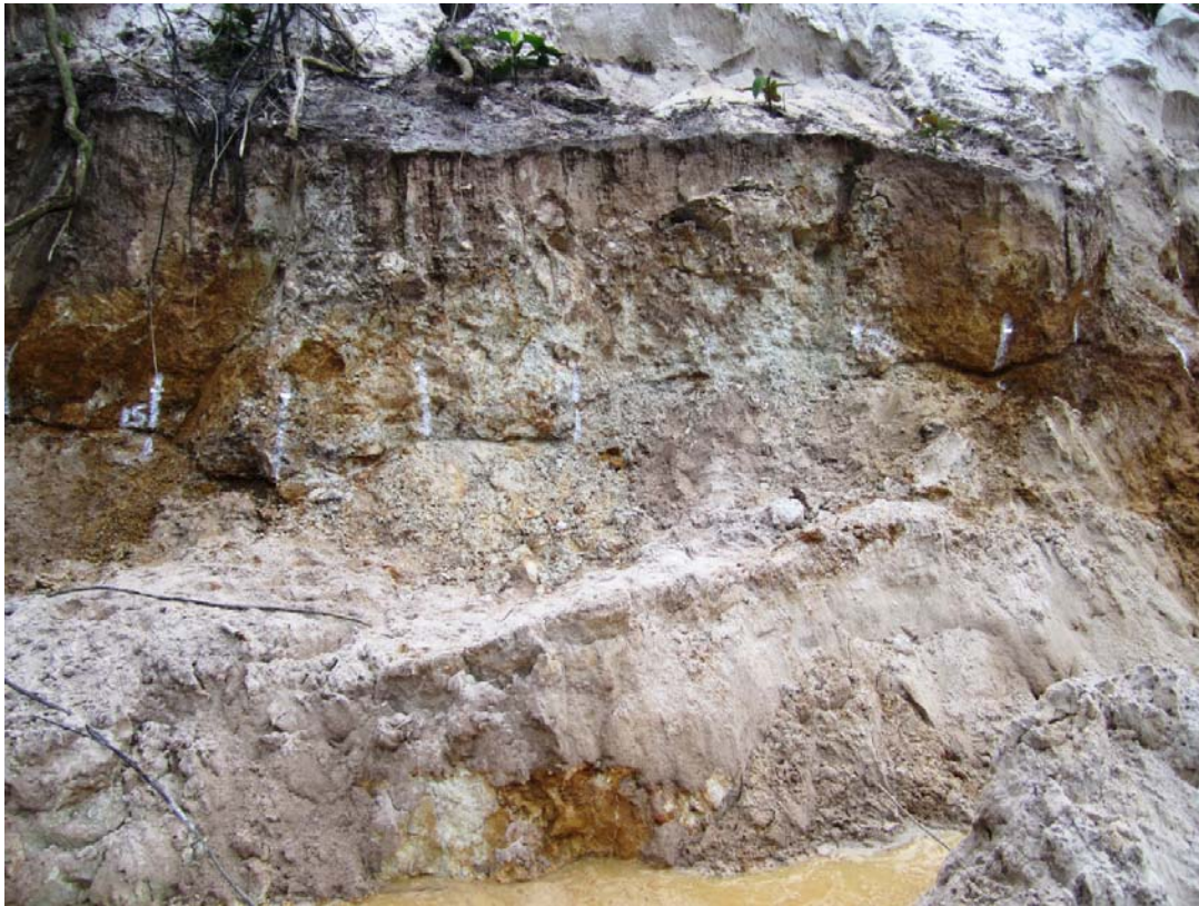
Figure 3 Five metre wide quartz - clay breccia zone, flanked by zone of intense quartz veining and limonitic relic sulphide development. White marks are spaced one metre apart.
