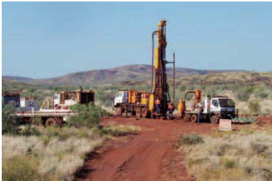
Fig 3 RC drilling at Marillana
