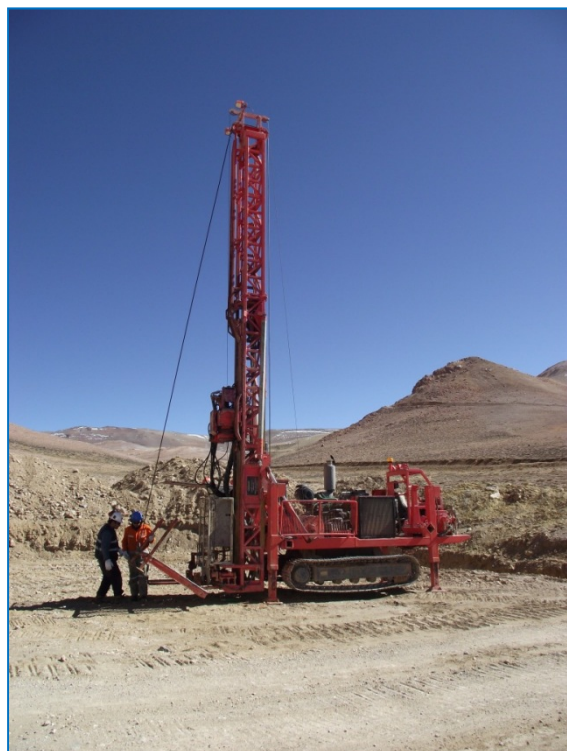
Figure 2. Preparing to drill geotechnical holes.
