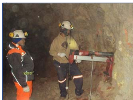
Hand-coring metallurgical samples from
