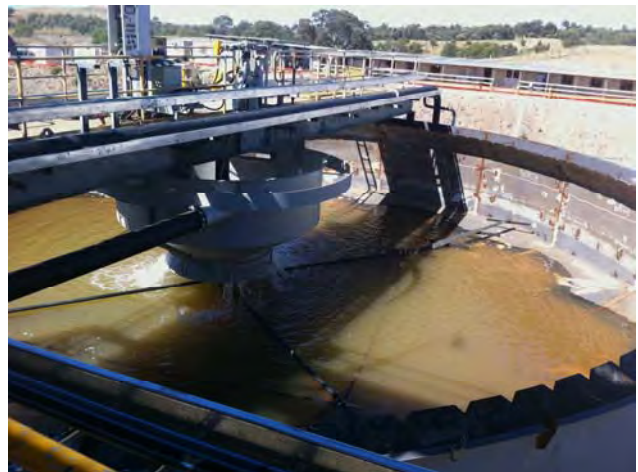
Tailings Thickener – wet testing
