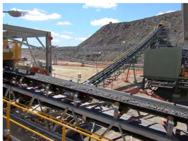
Clockwise: Ore being loaded into the Jaw Crusher, crushed ore on conveyor from Jaw to Secondary Crusher and through to ore stockpile
