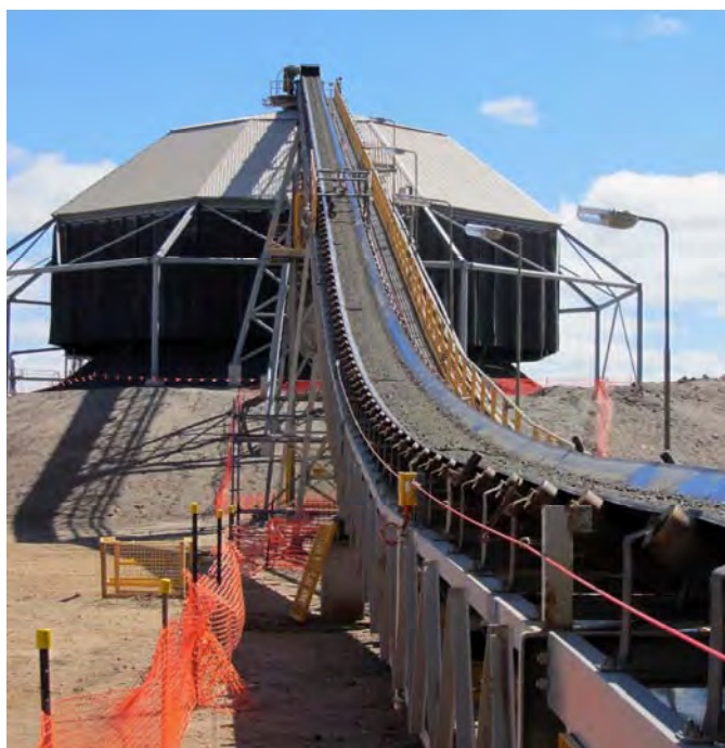
Clockwise: Ore being loaded into the Jaw Crusher, crushed ore on conveyor from Jaw to Secondary Crusher and through to ore stockpile
